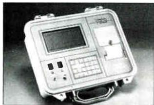
MTDR-Cable Fault Locator
