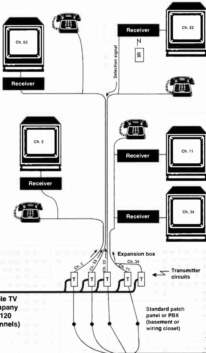
Goodman's favorite example of a possible application by cable operators is to use the system in a basement of an apartment building. There, the signals are fed to the telephone wires where they converge. Other possible applications include: transmission of a video signal from a VCR in one room of a house to a TV in another room; distribution of video signals in an office building for videoconferencing; delivery of signals from a fiber node to TV set-tops.
