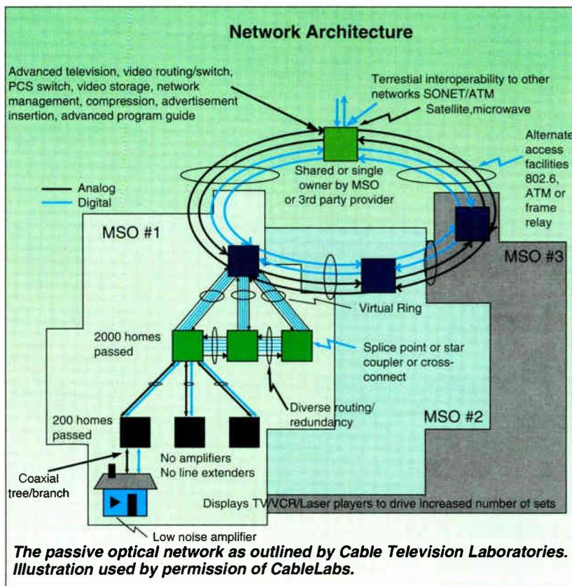
**The passive optical network as outlined by Cable Television Laboratories. Illustration used by permission of CableLabs.**
