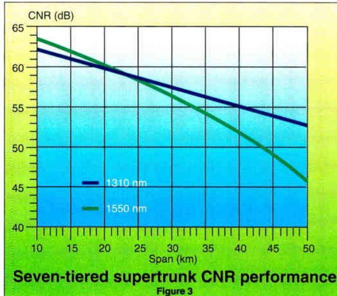
compare and contrast the 1310 and 1550 nm DFB laser diodes. For instance, the OMI at both wavelengths is close to their respective theoretical values shown in Table 1. The 1310 nm laser diodes were operated within a few percent of their OMI clipping point while the 1550 nm laser diodes were less than half of their clipping point. This difference is due to the dispersion-induced intermodulation distortion at 1550 nm. In
