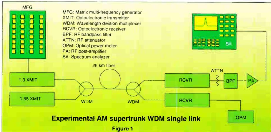
nm window in singlemode fiber because of its lower loss vs. distance profile and the technical capability to use optical amplification at this wavelength.
