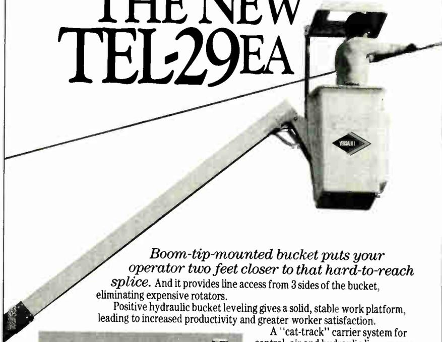
*Boom-tip-mounted bucket puts your operator two feet closer to that hard-to-reach splice.* And it provides line access from 3 sides of the bucket, eliminating expensive rotators.
