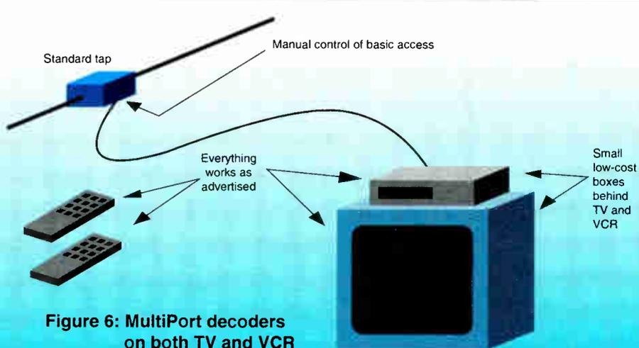
Figure 6: MultiPort decoders on both TV and VCR
