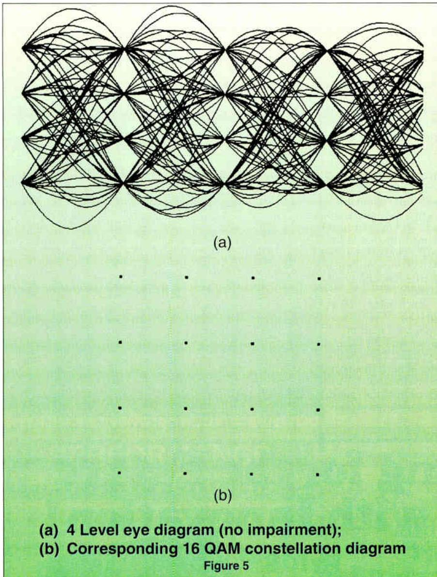
responding to each of the adjacent symbols time displacement from the present output point. The output of this module is two data files (I and Q) representing the analog baseband Nyquist waveforms sampled at 16 points per symbol. These files can be displayed graphically and independently as eye diagrams, or together as a constellation diagram using the Simulation Tools module, which is explained next.
