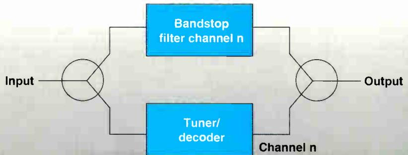
**Figure 4: Converter with bypass filter**
