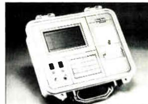
MTDR-Cable Fault Locator
