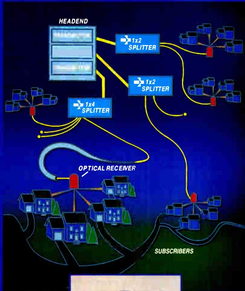
For CATV systems Gould has wavelength independent splitters with low insertion loss and high directivity ( $\leq -65.0\text{dB}$ ) -- guaranteed for environmental stability and performance at the headend or in the field. Components are in stock in a variety of standard and customized package styles.
