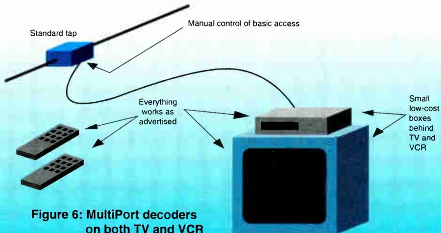
Figure 6: MultiPort decoders on both TV and VCR
