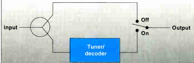
Figure 3: Converter with bypass switch
