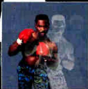
Test image with two multipath distortion echoes
