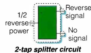
to prevent reverse signals entering one output from appearing at the other outputs.
