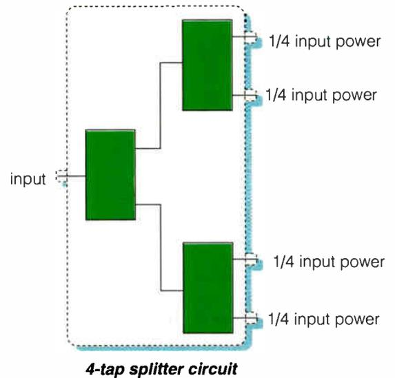
Ideal three-tap splitters have a -6 dB loss resulting from two of the taps to the input, while having a -3 dB loss from the remaining tap to the input. Ideal four-tap splitters have a -6 dB loss from any of the outputs to the input.
