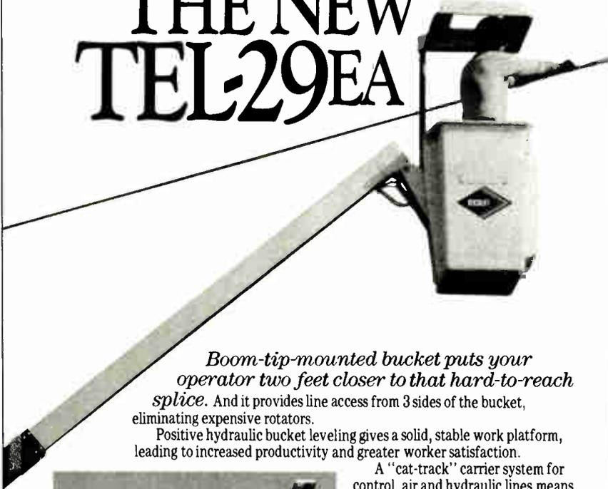
*Boom-tip-mounted bucket puts your operator two feet closer to that hard-to-reach splice. And it provides line access from 3 sides of the bucket, eliminating expensive rotators.*
