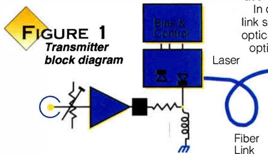
laser with no isolator. The transmitter consists of a return band hybrid CATV amplifier driving a FP laser. Resistive matching is used between the amplifier and the laser, though transformer matching has distinct advantages for return band transmitters. The use of transformer matching will be discussed later in this paper.
