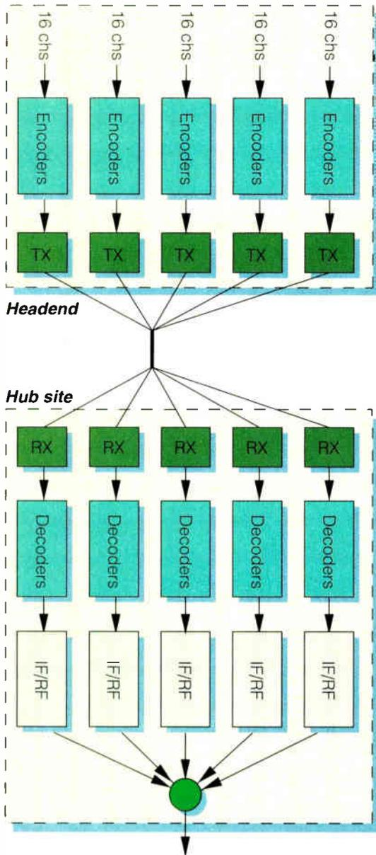
An 80-channel digital system with RF outputs typically requires no more than one six-foot rack at the headend and about two seven-foot racks at the hub site. The digital transmit and receive equipment requires an environmentally controlled building.
