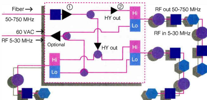
The pure passive network presents a power system designer with an interesting proposition. Because the fiber optic receiver represents a last active device in the "ideal" PCNA, there is no requirement to transmit power through the coaxial distribution network.
