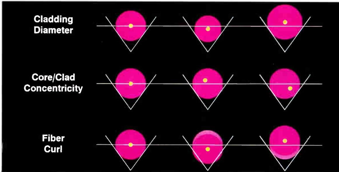
same size, helping to avoid core offset in mechanical joining. These tolerances are controlled during manufacture by draw rate (how fast a fiber is made) and temperature. On-line, in-process computer controls measure the fiber's diameter hundreds of times per second, as a closed-loop system continuously monitors and adjusts the fiber draw process.
