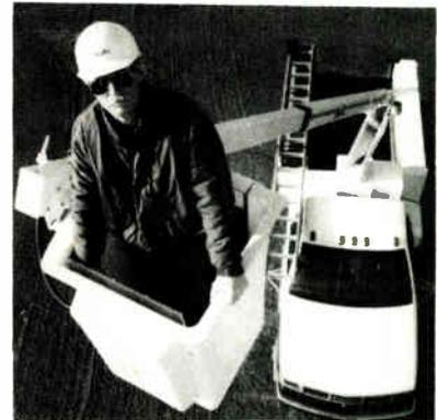
valve at tank and/or bucket allows operator to bring down the boom in the event of power failure. Hydraulic and electrical lines are enclosed inside the boom and a friction lock prevents tipping of gravity leveled buckets.
