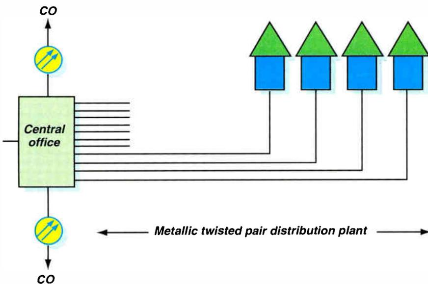
Figure 1b: Fiber and twisted pair switched circuit network
