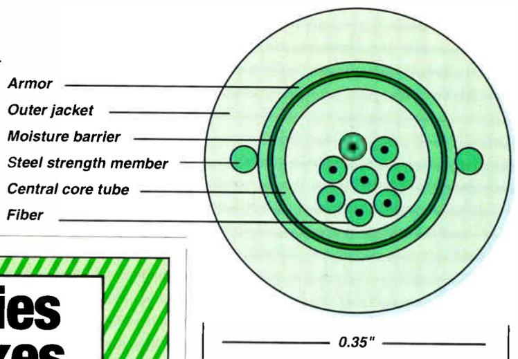
**Broadband Distribution Cable**—Exact number of fibers will be dictated by the network. For a broadband switched circuit fiber to the node architectures the number of fibers will most likely be between two and ten fibers.
