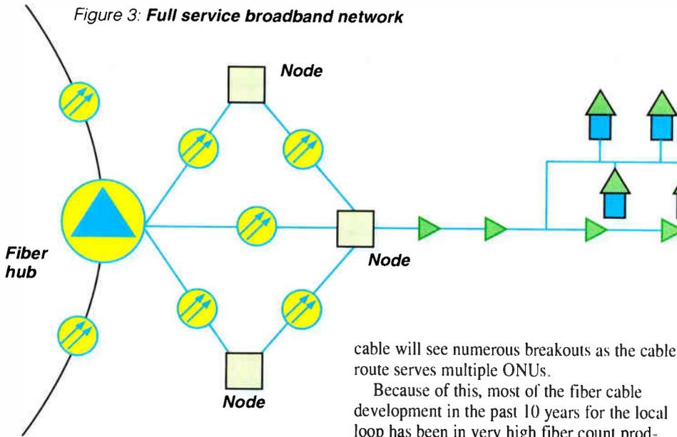
(subscriber loop). To put fiber optic cables in a dedicated line subscriber architecture requires cable with high fiber counts. This is seen by looking at how a single distribution fiber cable in Figure 1B is used to feed multiple ONUs after it leaves the HDT. One leg of
