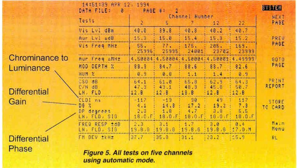
Figure 5. All tests on five channels using automatic mode.
