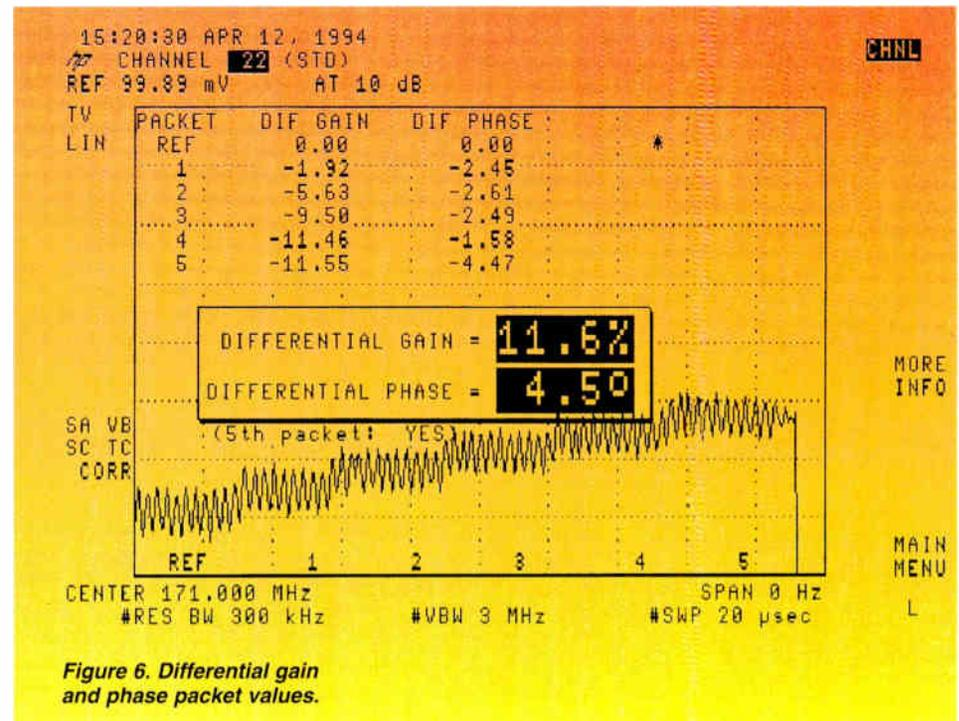
Figure 6. Differential gain and phase packet values.
