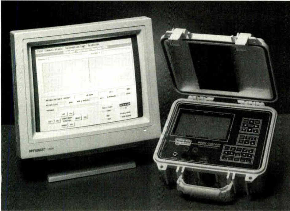
**Riser-Bond's 1205T time domain reflectometer**
