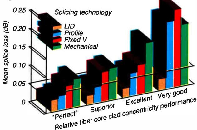
However, cable TV operators can control their splicing costs by understanding and influencing the major variables that impact splice costs. Although external variables like fiber handling and splicing-area cleanliness play a significant role in splicing, we have focused on, for the purpose of this paper, the
