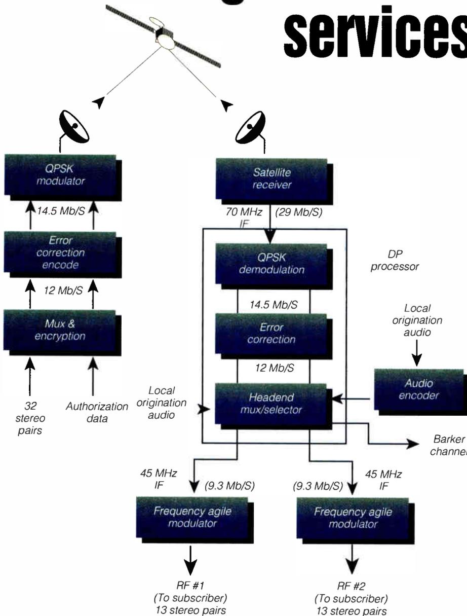
Figure 1: Basic DP transmission link
