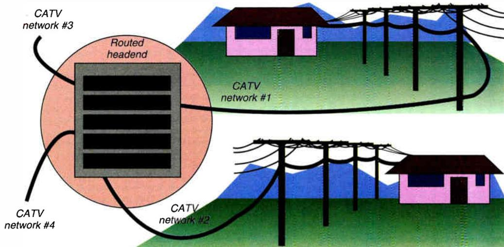
**Figure 3:** Treating each CATV trunk as a segmented network allows traffic to be controlled at the headend router. In this way, eavesdropping and theft of service exposure can be limited to a specific trunk, and hackers can be detected and blocked.
