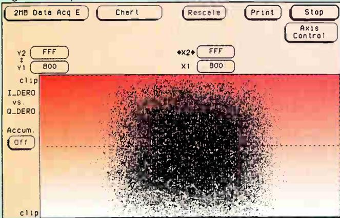
Figure 4: Equalized 256-QAM constellation
