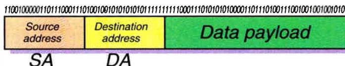
Figure 1: The Ethernet data packet. The Source Address (SA) of the Ethernet packet can be used to make decisions on access to the network and can be used to indicate an unauthorized transmission.
