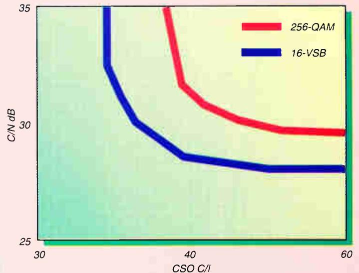
Figure 3: Phase noise & white noise threshold
