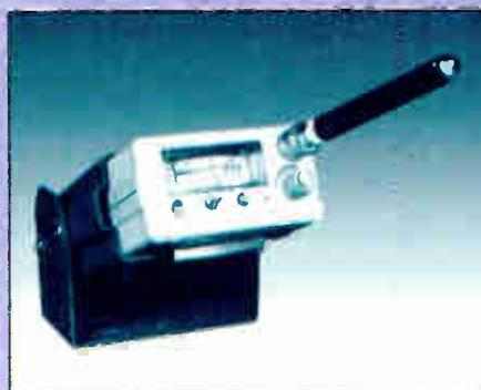
**Searcher Plus** Performs calibrated leakage measurements down to 2 microvolts per meter. Comes with mobile mount for quarterly driveouts, and can be hand-carried to pinpoint leak source.
