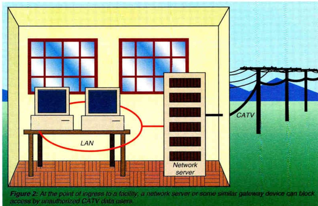
Figure 2: At the point of ingress to a facility, a network server or some similar gateway device can block access by unauthorized CATV data users.
