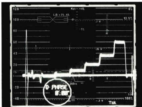
Figure 4: This is the waveform monitor single trace diff phase indicating 6 degrees of differential phase distortion.
