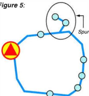
the unit to provide primary and backup two-way digital traffic in the event of a fiber cut.
