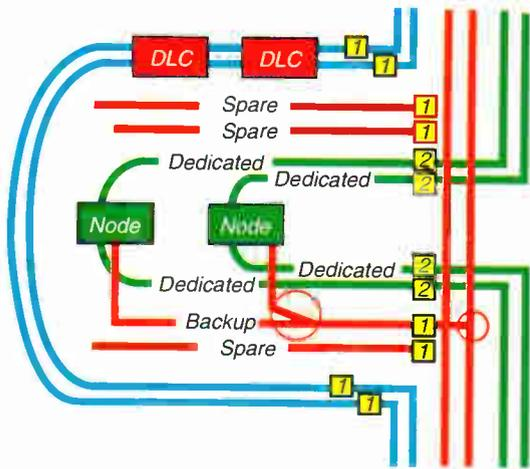
associated with CATV, such as IPPV and interactive game signals in an integrated manner. The DLC/Sonet technology may be adapted to meet these additional requirements, or perhaps other transport methods may become available. In any case, the Ring-in-Ring architecture is flexible enough to accommodate whatever the integrated solution or solutions may be.
