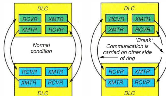
Figure 3: SONET Digital Loop Carrier. Possible equipment configuration
