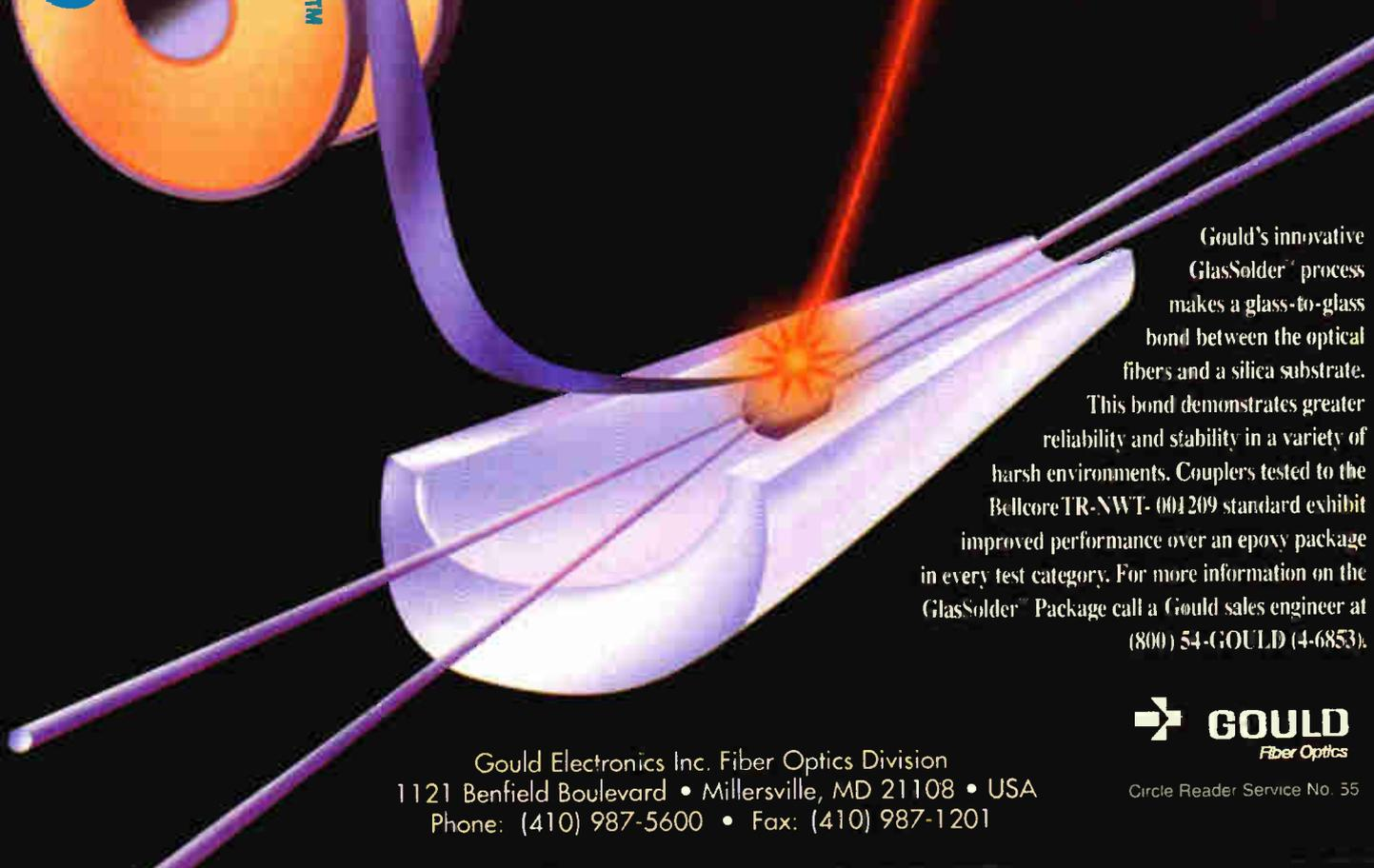
Gould's innovative GlasSolder™ process makes a glass-to-glass bond between the optical fibers and a silica substrate. This bond demonstrates greater reliability and stability in a variety of harsh environments. Couplers tested to the Bellcore TR-NWT-001209 standard exhibit improved performance over an epoxy package in every test category. For more information on the GlasSolder™ Package call a Gould sales engineer at (800) 54-GOULD (4-6853).
