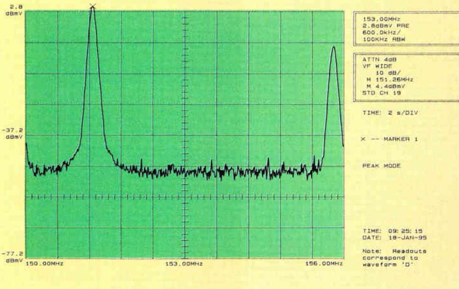
Typical gated spectral presentation of a channel in service. We have "gated out" the video signal to create a clear view of the in-band noise.
