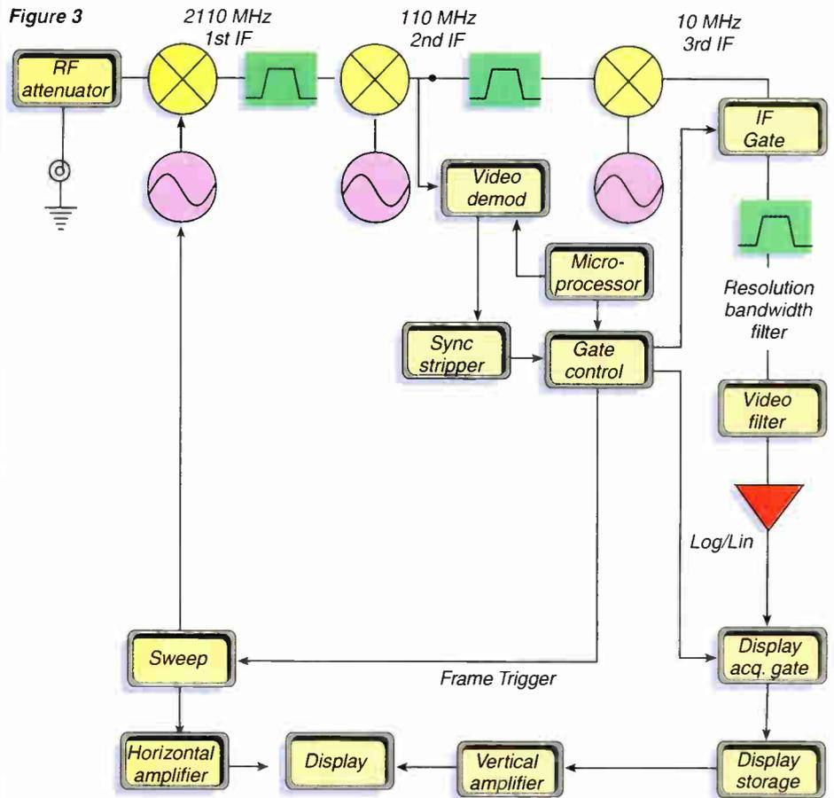
Signal path for gated measurements.
