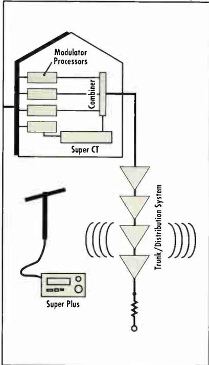
Trilithic's channel tag system is easy to install - just place it in series with your modulator or processor output. It emits its marker signal over an existing carrier - eliminating the need for a separate test frequency.
