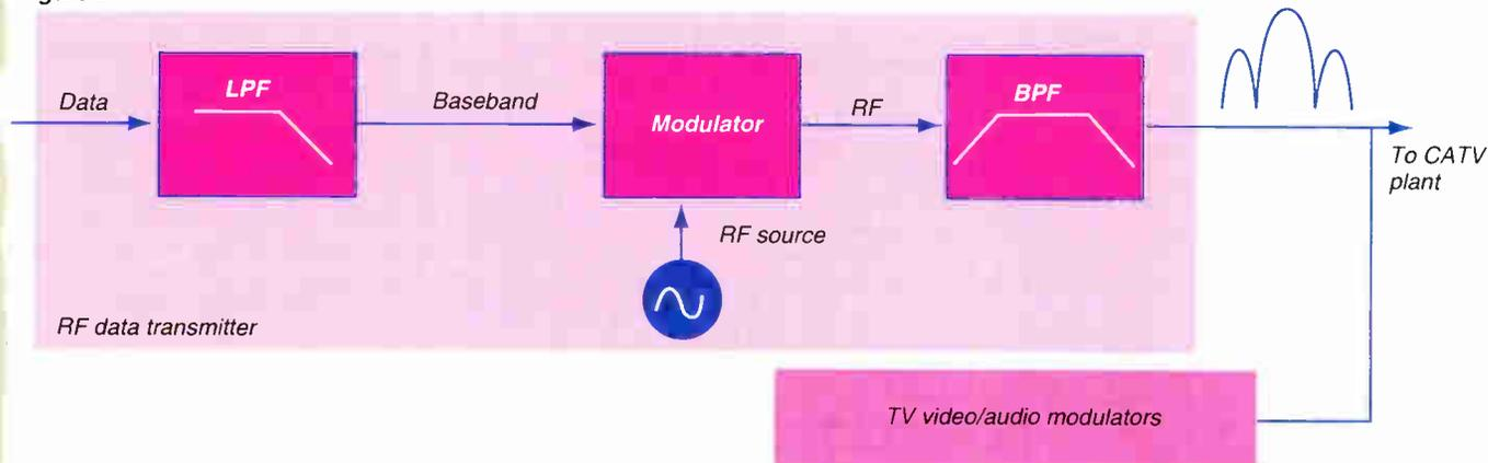
include BPSK, QPSK and QAM. Each modulation scheme has an associated RF bandwidth efficiency which is typically described in terms of bps/Hz, where the system bandwidth is assumed to be the Nyquist RF bandwidth. Note that the Nyquist RF bandwidth is twice as wide as the Nyquist baseband bandwidth for double-sided modulation schemes. For example, BPSK modulation can support 1 bps of NRZ data for each 1 Hz of transmitted RF
