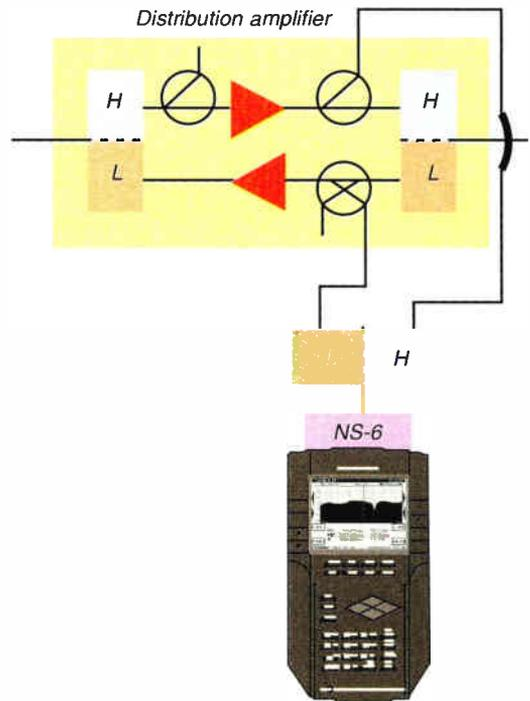
telemetry and sweep, as well as inject reverse telemetry and sweep. This summing network simplifies the connection of the field receiver to the test point.
