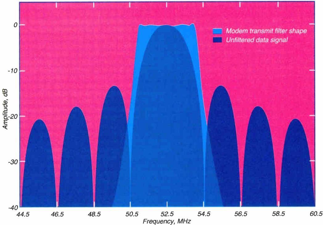
adjacent spectrum. Nonetheless, out-of-band energy may spill over into adjacent channels due to non-ideal filtering. This energy may introduce an interfering signal to adjacent television and/or data channels, and may degrade the carrier-to-noise ratio of the adjacent televi-
