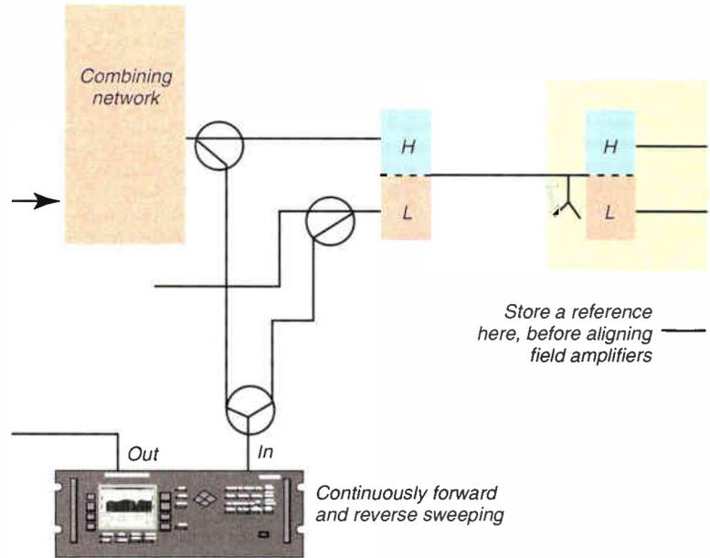
sweep. One handheld instrument in the field does both the forward and reverse sweep tasks, eliminating the need to carry multiple boxes. The reverse option has the capability to sweep return with up to 250 kHz resolution, ensuring that no response problems are overlooked.
