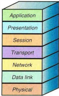
In the case of an HFC network, the Physical Layer includes the headend equipment and the distribution components. It also includes the equipment at the user site, commonly called a "cable TV modem," which converts the digital information into a modulated RF signal and demodulates it back to digital information.
