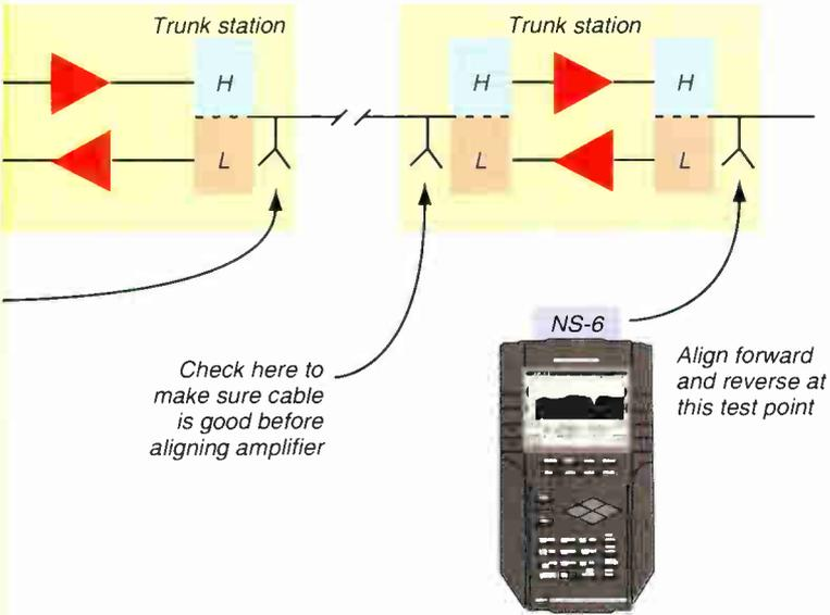
signal that indicates which receiver is sending the sweep. The headend transmitter measures the sweep, and sends the results, along with the serial number of the sending receiver, via its telemetry signal to the field. The field receiver with the tagged serial number then displays the sweep response as measured in the headend on its LCD.
