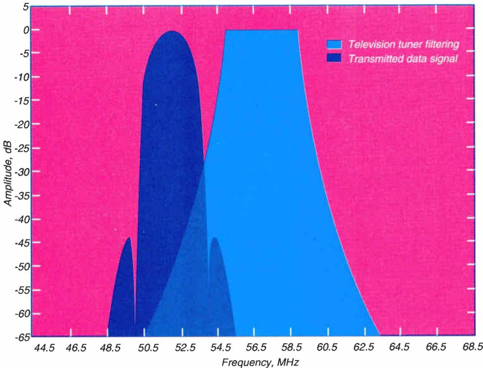
culated by integrating the residual sidelobe power over the bandwidth of the television channel. This average interference power is then added to the noise floor to determine the resulting carrier-to-noise ratio.
