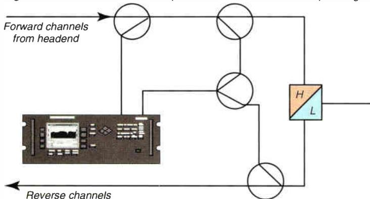
Figure 2: Headend transmitter setup with reverse node combiner (multiple node returns)
