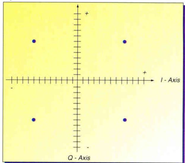
this ratio is decreased, the picture quality as viewed from a video monitor starts to degrade. The requirements of the QPSK modulation technique used for data transmission is >30 dB carrier-to-noise measured over 6 MHz. This is not an issue because noise tends to be broadband in nature, and if the carrier-to-noise ratio is being met and kept for video transmission, then data is able to run in this same environment without problems.
