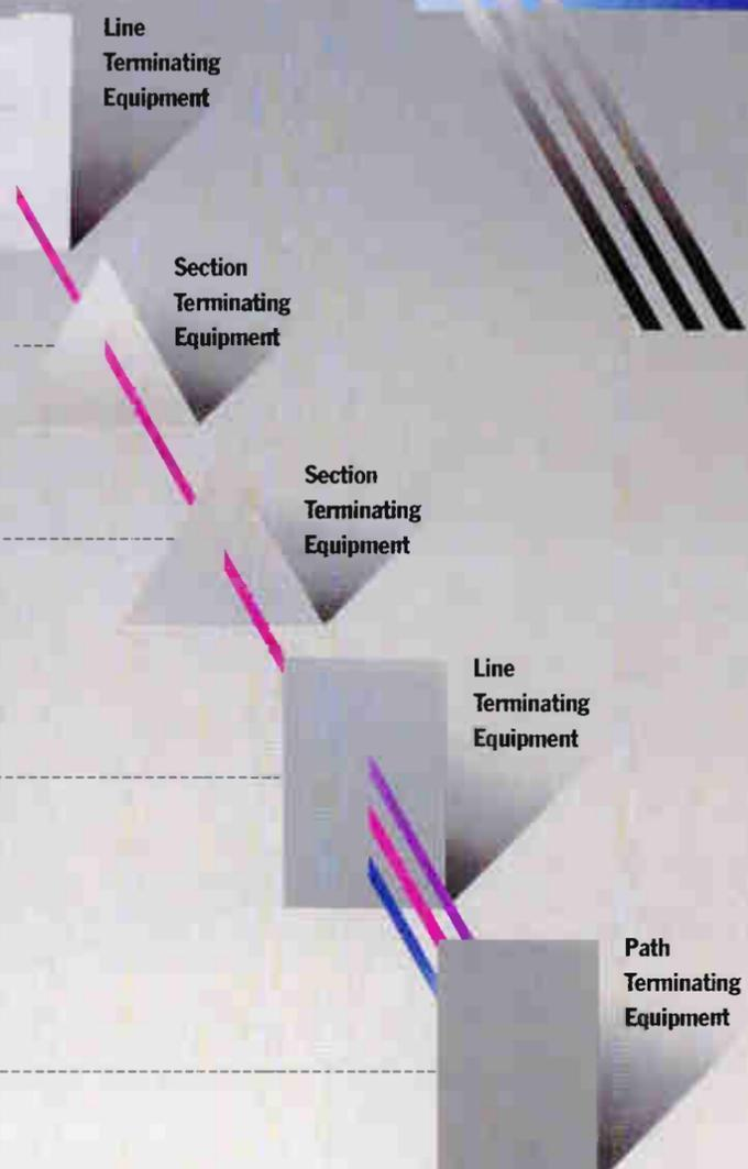
**Line Terminating Equipment (LTE).** Network Elements (NE) that originate and/or terminate line (OC-N) signals. LTEs can originate, access, modify, or terminate the transport overhead, or can perform any combination of these actions.
