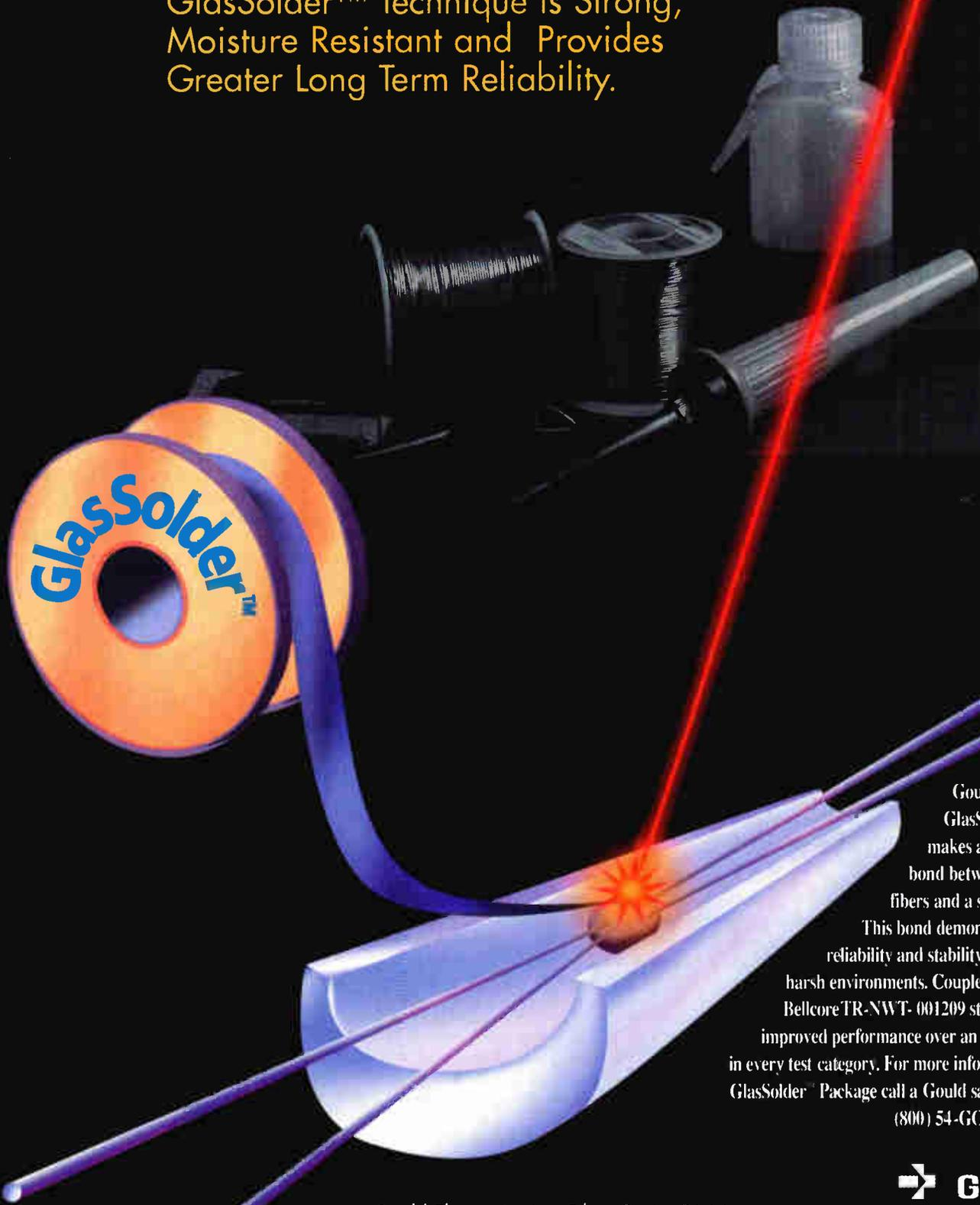
Gould's innovative GlasSolder™ process makes a glass-to-glass bond between the optical fibers and a silica substrate. This bond demonstrates greater reliability and stability in a variety of harsh environments. Couplers tested to the Bellcore TR-NWT-001209 standard exhibit improved performance over an epoxy package in every test category. For more information on the GlasSolder™ Package call a Gould sales engineer at (800) 54-GOULD (4-6853).
