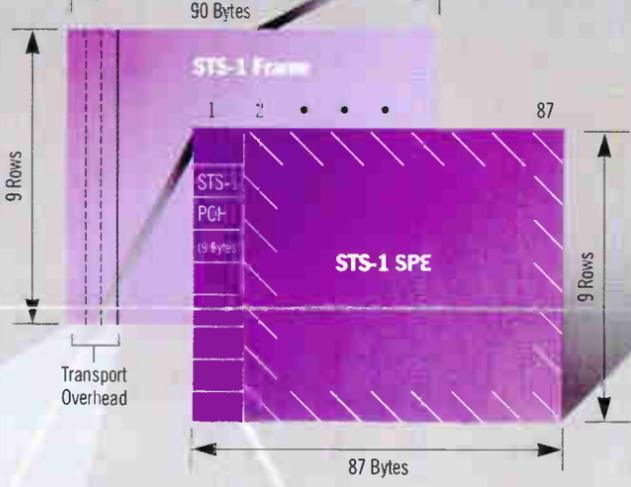
Synchronous Transport Signal level 1 (STS-1). Basic logical building block signal with a rate of 51.840 Mbit/s.
