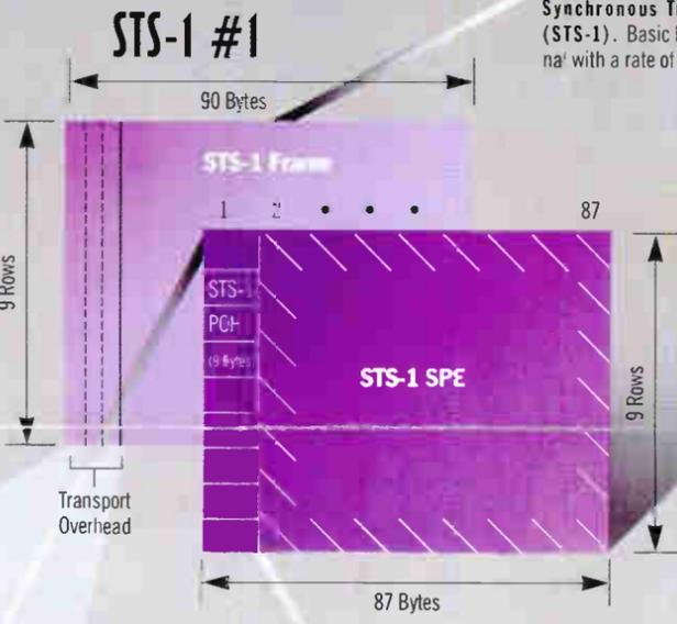
Synchronous Transport Signal level 1 (STS-1). Basic logical building block signal with a rate of 51.840 Mbit/s.
