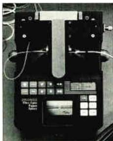
**Fusion 2000, an automatic fiber splicer**
