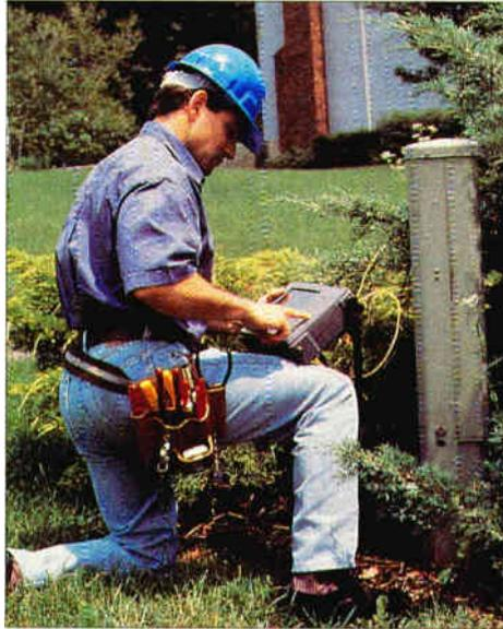
**MW9070A mini-OTDR, with MW0972 module**
