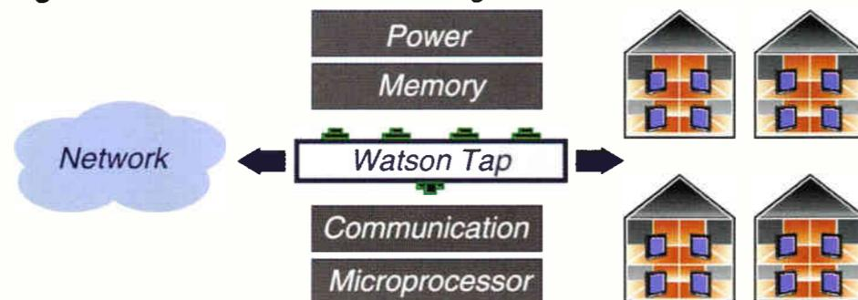
reducing unauthorized programming use, increasing the viewer's freedom of selection to an a la carte basis, and allowing for transactional based billing. The off-premise broadband controller provides a secure "in-the-clear" signal transmission path of programming into the home, thereby eliminating the cable-consumer equipment incompatibility problem.
