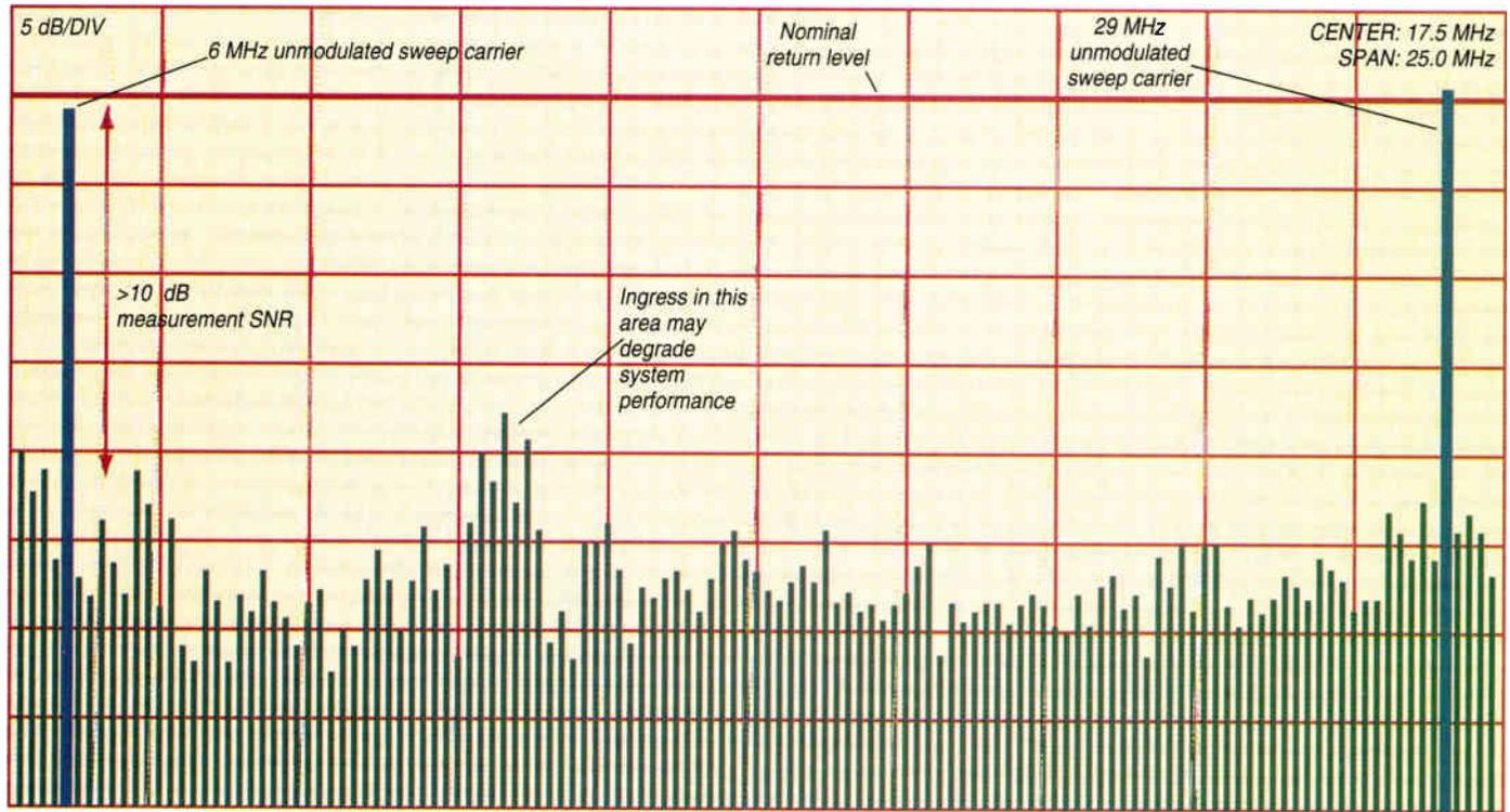
is receiving the proper upstream signal levels.
