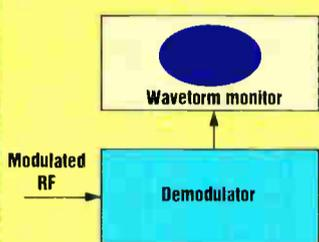
program video being measured, use 2 milliseconds/division and 60 Hz line sync to display one field.
