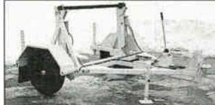
The trailer has a capacity of 2500lbs., with reel dimension capacity of 72" diameter (96" optional), and 60" width. Options available: electric hydraulic power, anti-backlash brake, tool boxes, chocks and holders.
