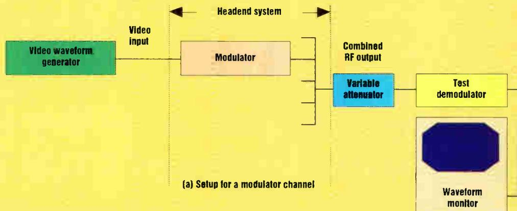
(a) Setup for a modulator channel
