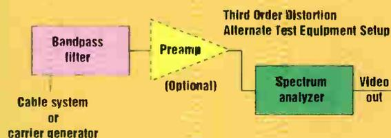
2. Adjust analyzer center frequency to peak the set-top's visual carrier output.
