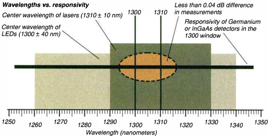
**The difference in responsivity between 1300 and 1310 nm for most optical power meters is less than one percent.**
