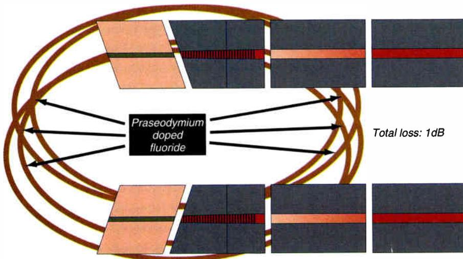
Having developed a suitable fluoride fiber, the next obstacle was developing a means to provide this fiber in a package compatible with silica fiber. This was not an easy task, considering that fluoride and silica fibers have such dissimilar characteristics. The key issues are illustrated in Figure 1. For amplification purposes, the fibers need to be spliced in a way that supports optical transmission in both the 1310 nm band and in the band of the pump frequency.
