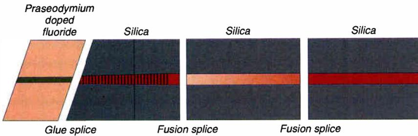
the results of their research. Using a single praseodymium doped fluoride fiber amplifier (PDFFA), they generated 16 dB of amplification in the optical domain and transmitted a 5 Gbps data stream at 1310 nm over 100 km of silica cable. While BT's experimental results demonstrated a technical solution, providing the telecommunications industry with a practical PDFFA required more creative research and engineering.
