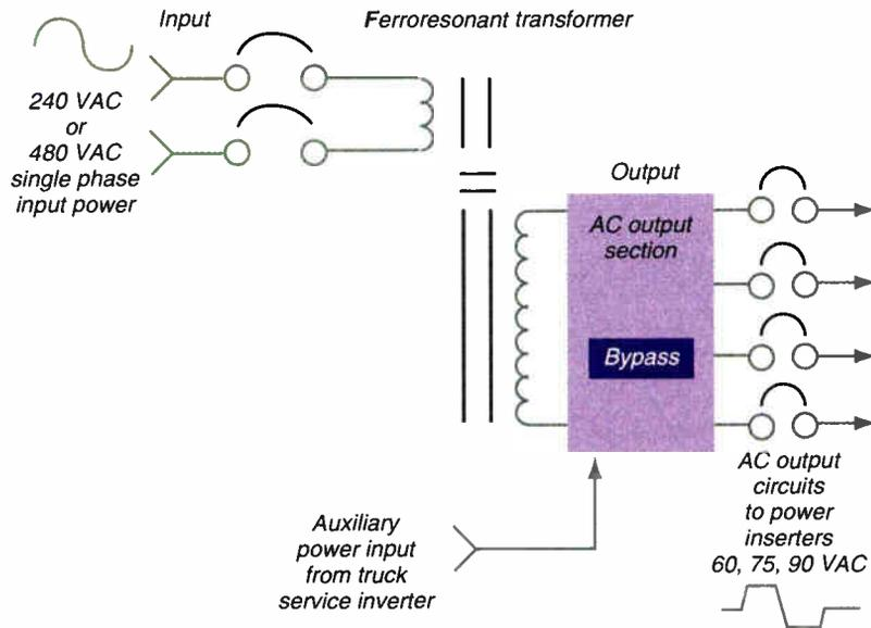
down the coax to the RF amplifiers, fiber nodes, network interface units and telephony equipment, SNET selected conventional 60- and 90-volt, 60-Hz, quasi square-wave power.
