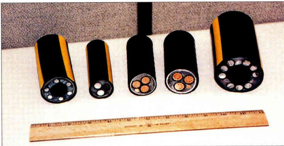
View of the various cable types used in the construction of the overall system. From the left, the cables are: six conductor branch cable with innerduct used for side branches, two conductor branch composite cable used for single node branches, 2/0 copper CLX used in underground ducts, 4/0 copper CLX used in underground ducts and nine conductor feeder cable used in primary aerial backbone.
