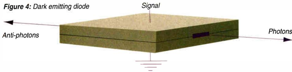
either praseodymium or neodymium for operation at 1310 nm. Photons are emitted at the front facet, which is the normal facet for signal collection. Anti-photons are emitted out the rear facet, and for the purposes of impulse control, this is the facet that is connected to the fiber. This fiber is combined with the signal fiber, and the resulting cancellation is fed to a normal fiber receiver.
