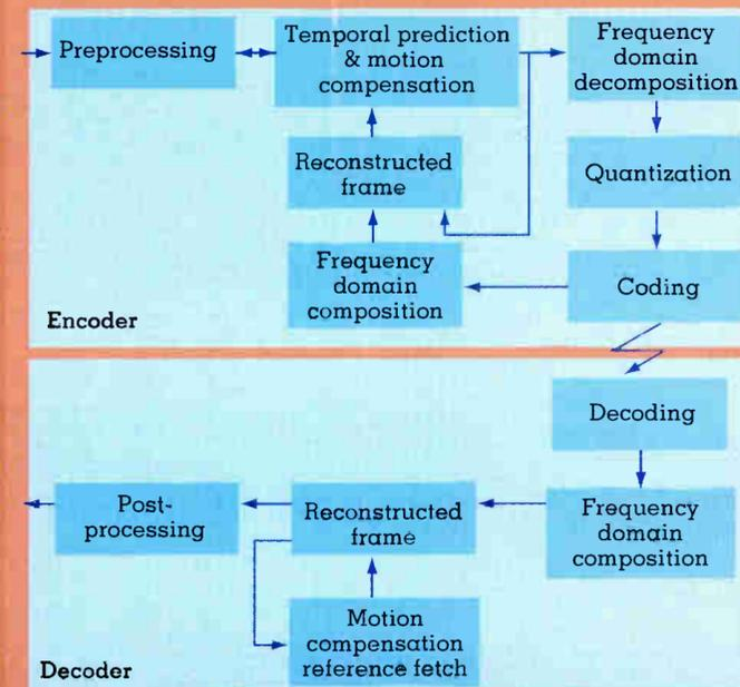
actually code only the changes that occur from one frame to another. This is known as "interframe" coding. Sending information only about the changes dramatically reduces the amount of data that has to be transmitted. In the MPEG process, bidirectional prediction is used to help forecast motion. This step buffers several frames so that the preceding and succeeding images can be examined and compared to determine how much motion takes place and where the moving objects should be placed.
