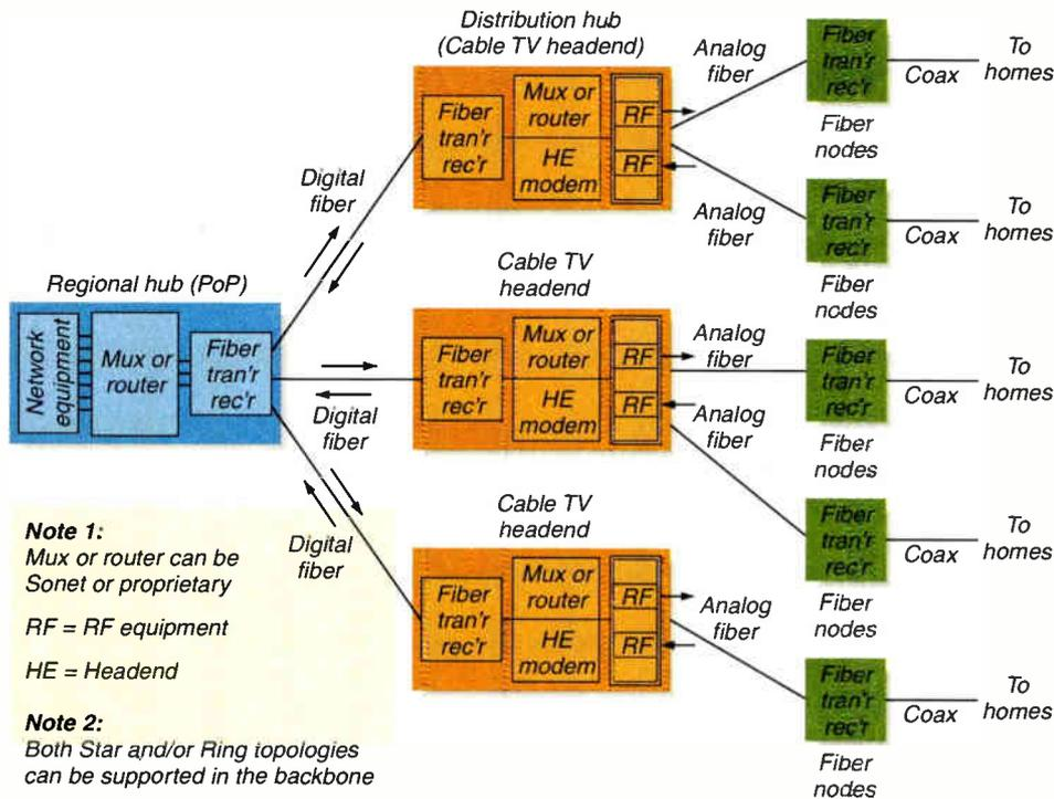
Figure 3: A typical MAN with digital transport and HFC distribution
