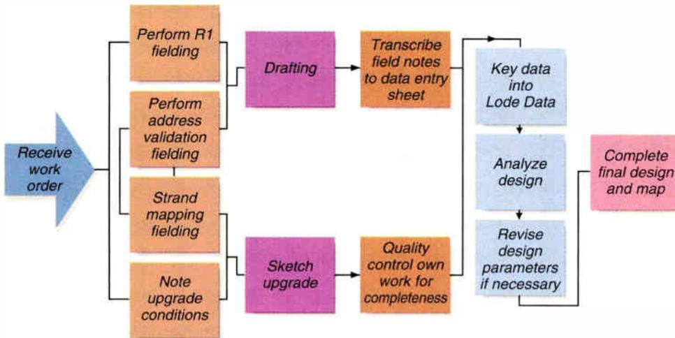
fielding at D&A. R1 fielding takes place before MDU fielding—an R1 fielder works independently, measuring trench footages, estimating drop footages, recording house counts, recording device descriptions and noting discrepancies (areas where the equipment is damaged or the system is not up to current specs
