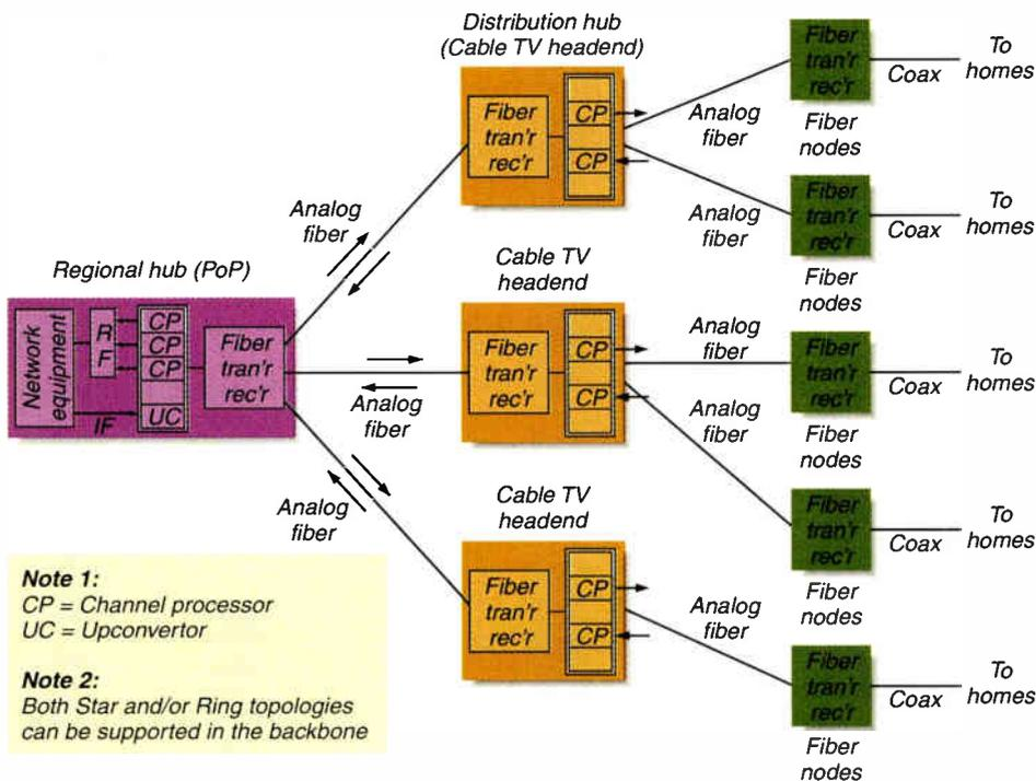
Figure 2: A typical HFC MAN for both transport and distribution
