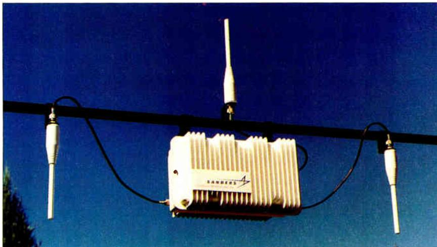
*This Cable Microcell Integrator (CMI) transceiver was designed and built by Sanders Telecommunications Systems to provide the air-to-cable interface for a cable TV-based implementation of Personal Communications Services (Photo courtesy of Sanders).*
