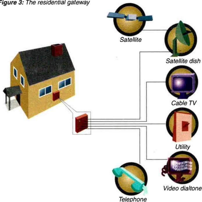
with high bandwidth “digital” services, such as Internet access, HDTV and services yet to come. The RG approach provides this intelligent interface and has many inherent advantages.
