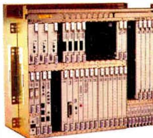
**The FACTR® platform supports broadband and narrowband services from a single mechanical package.**
