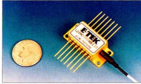
**1550 nm laser diode power module**
