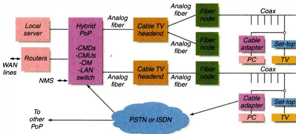
Figure 5: The two most popular SCAN configurations
