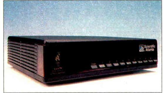
***S-A will provide 6,600 of its 8600X Home Communications Terminals for the Games. The 8600X will be used to select among 48 video channels, and up to 100 Press Data Channels available on the system.***
