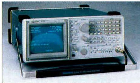
Tektronix' 2715 Cable TV Spectrum Analyzer
