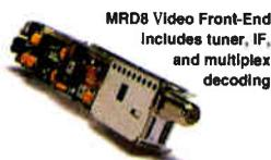
MRD8 Video Front-End includes tuner, IF, and multiplex decoding
