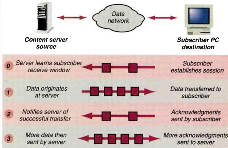
When a network and subscriber PC are fast, TCP acknowledgments are transferred quickly (with low latency or delay) to the content server, enabling a rapid data transfer. If either the subscriber PC or interconnecting network is slow, (due to either a low throughput downstream or high latency upstream) the content server will slow the transmission rate to a more acceptable level, one that does not cause network congestion or overrun the subscriber PC receive rate.
