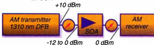
fiber Bragg grating filter is used to block the 1290 nm emission, a highly linear 10 to 15 dB fiber-to-fiber gain around 1310 nm is obtained.
