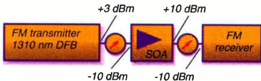
However, when an SOA is inserted in the signal path, the amplified spontaneous emission (ASE) of the laser, along with the Rayleigh backscatter feed-back into the FP laser, increase the laser noise and affect its performance. Further work needs to be done to identify this problem precisely and to propose a cost-effective solution.
