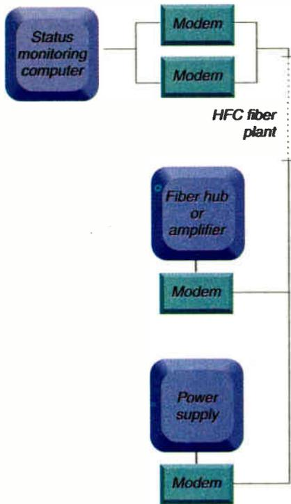
analog, and are translated into digital form and transported from the measurement point to the operations center. Transport is accomplished through the RF modem upstream over a return cable. Frequencies for transport are chosen according to the system design, and may be in the sub-, mid- or high-frequency range.
