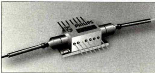
Figure 1. Illustration of a fully packaged semiconductor optical amplifier.
