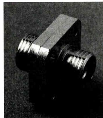
**A bulkhead fixed “coupling” attenuator (FC compatible) is easily installed between two patch-cords to provide (typically) 5, 10, 15 or 20 dB of attenuation. Also available in SC or ST styles.**
