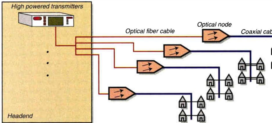
Figure 6: HFC network narrowcast transmission platform (field upgradable to narrowcast)
