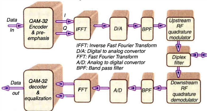
Figure 2: Modulation Efficiency and ingress protection.
