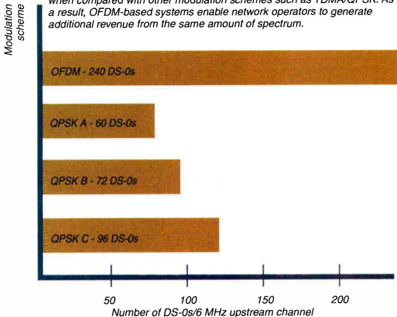
ciency. Studies have shown that typical interferers are in the range of 5 to 29 kHz wide, which would disrupt only one or two DS-0 channels, each 18 kHz wide. So this ability to move channels to different frequencies is a significant advantage.
