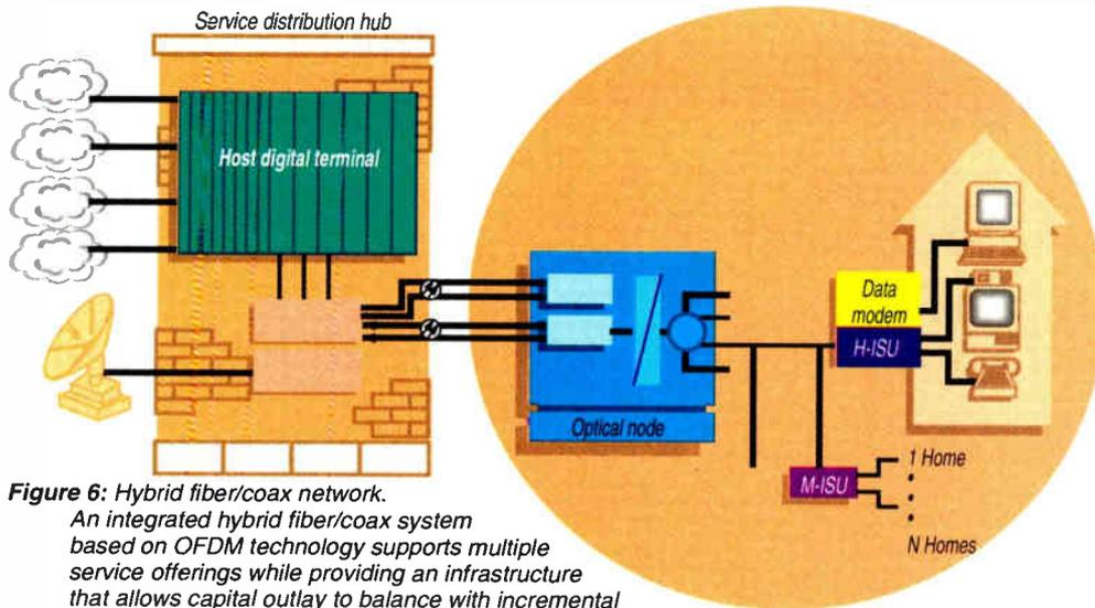
**Figure 6: Hybrid fiber/coax network.**
