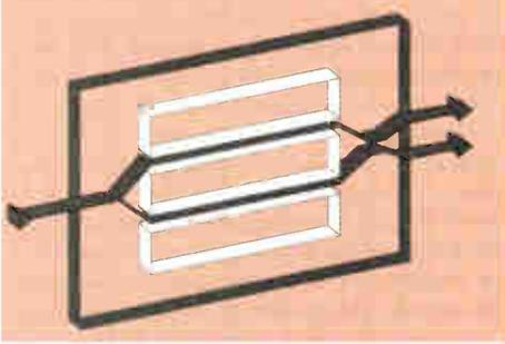
A second important component of this platform is a planar wave device used to optically split the raw optical power of the laser. Since each of the optical outputs is individually modulated, the number of transmission paths is determined by the planar waveguide divider. The device can be configured to provide between two to 16 divisions of the optical source, which will vary the optical output between levels. Each division is then modulated.
