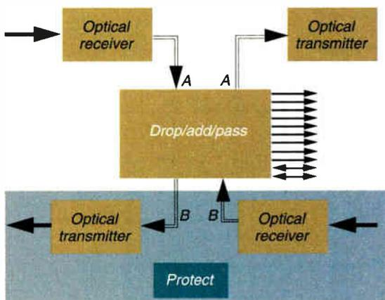
Figure 8: Universal uncompressed network with optical protective switching
