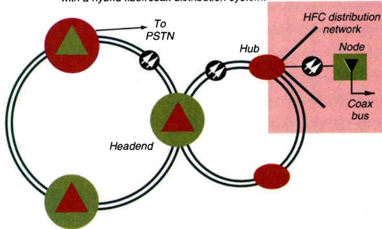
spectrum by replacing coax plant with higher bandwidth optical fiber and by greatly reducing the number of active RF devices the signal must pass through on its way to the end user.
