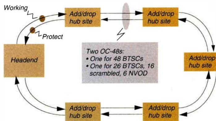
Figure 2: Example Sonet network equipment detail
