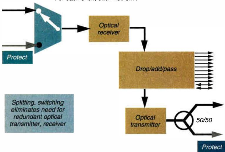
automatic protective switching for self-healing networks: Electronic (redundant optics) and optical. The system works with two types of network managers, including a TL-1 compatible system.
