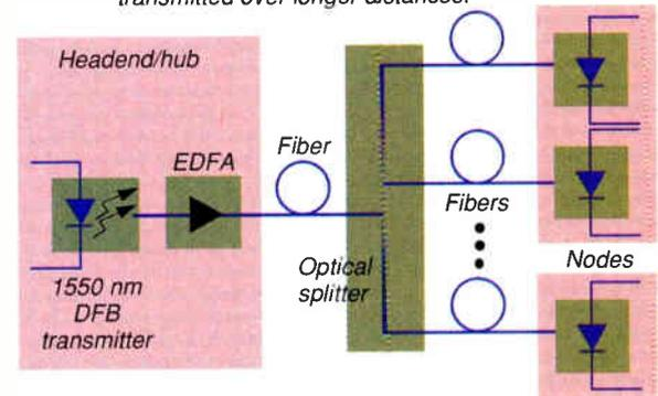
a fiber link will perform optimally with today’s single wavelength 1550 nm systems, as well as tomorrow’s dense wavelength-division multiplexing technologies.
