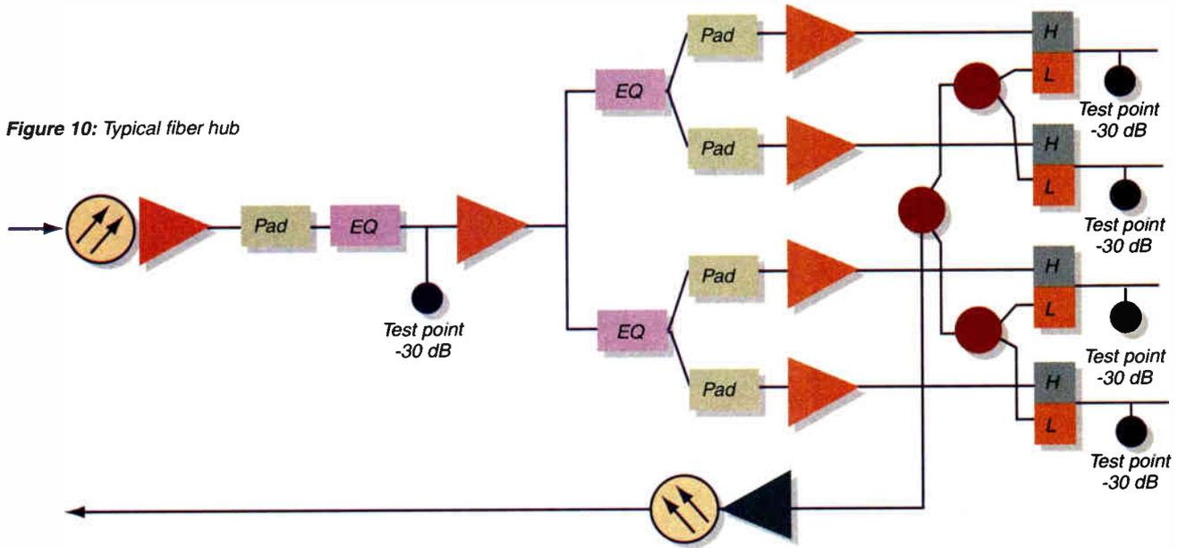
It is important to be familiar with the amplifier and fiber optic block diagrams (see Figure 10). Internal coupling and test point variations determine the loss between the sweep insertion point (IP) and the input to the amplifier or laser. In our experience, not having this information has been a major contributor to alignment problems.
