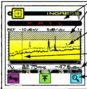
Limit with pass/fail indicator simplifies test for installers.
