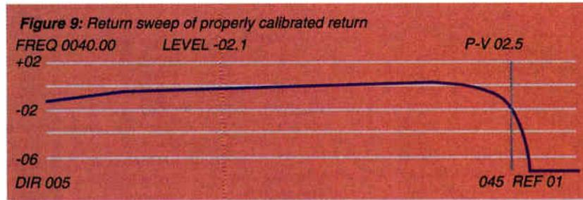
the fiber node return laser. When choosing this reference input level, consideration must be made for low-end optical and RF noise floors, as well as high-end clipping resulting from overdrive. A typical manufacturer's specification for
