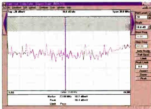
Figure 5: Ingress with a common path distortion component as displayed on a common PC-based analysis software package.
