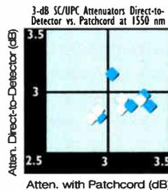
Consistent attenuation is achieved either with patch cables or when connected directly to the detector. The attenuator element does not strongly guide cladding modes that would produce different loss values when connected with or without a patch cable.
