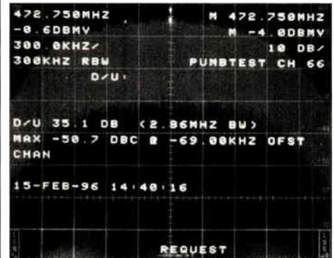
Figure 1: Tektronix's 2715 spectrum analyzer gauges desirable/undesirable (D/U) signal ratio on a digital channel.
