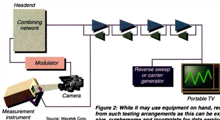
Figure 2: While it may use equipment on hand, results from such testing arrangements as this can be expensive, cumbersome and incomplete for data services.
