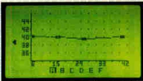
When equipped with the Multiplexer Option, the 9580SST accepts signals from up to 8 separate test points and analyzes sweep & ingress from each individually, returning data to as many as 6 SSR field units (A thru F) connected to it.
