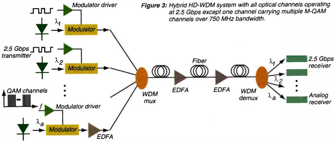
Figure 3: Hybrid HD-WDM system with all optical channels operating at 2.5 Gbps except one channel carrying multiple M-QAM channels over 750 MHz bandwidth.
