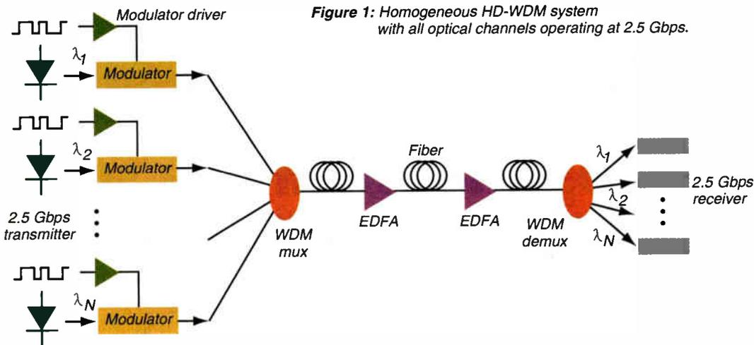
Figure 1: Homogeneous HD-WDM system with all optical channels operating at 2.5 Gbps.
