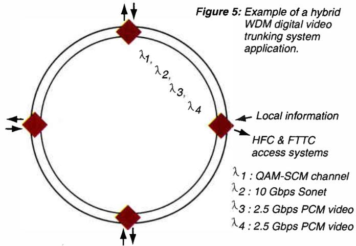
Figure 5: Example of a hybrid WDM digital video trunking system application.
