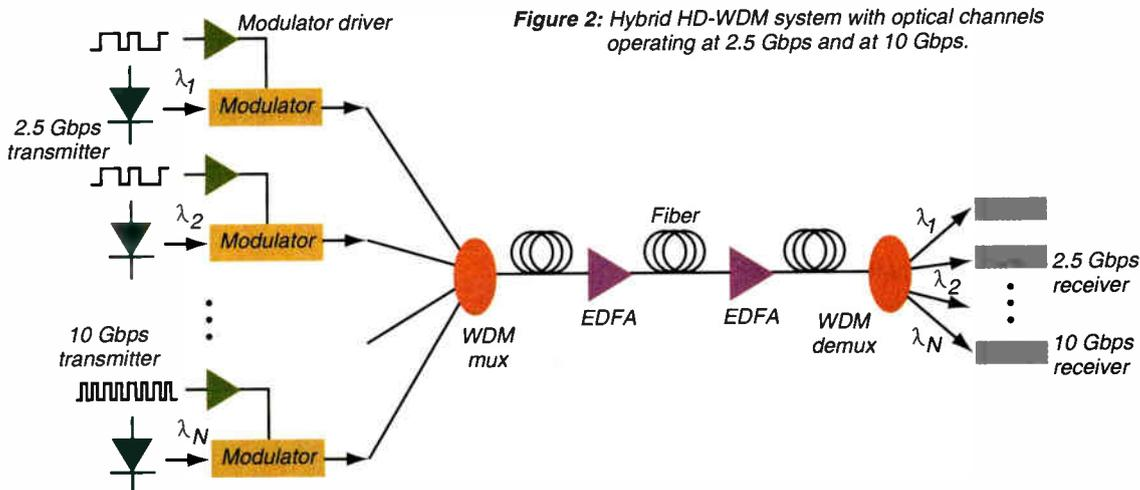
Figure 2: Hybrid HD-WDM system with optical channels operating at 2.5 Gbps and at 10 Gbps.
