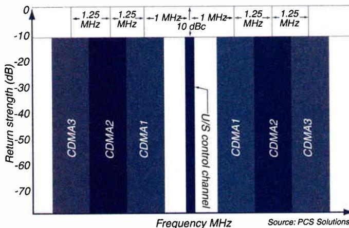
Figure 3: Upstream signal allocation.
