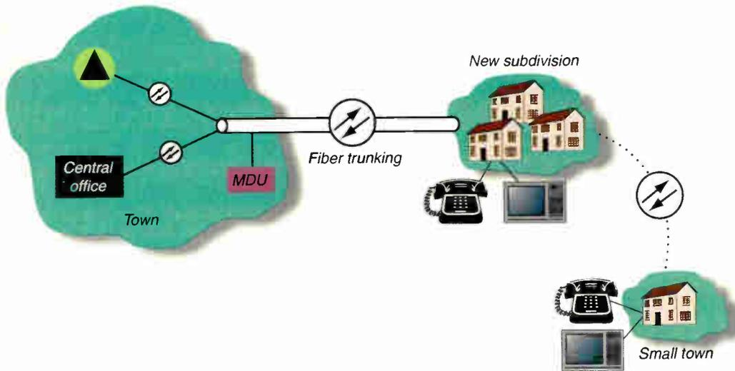
nant cost factor is the cost of fiber from the headend to the rural community, while other costs, such as optoelectronics for signal trunking, coaxial and twisted copper pair plant, are secondary.
