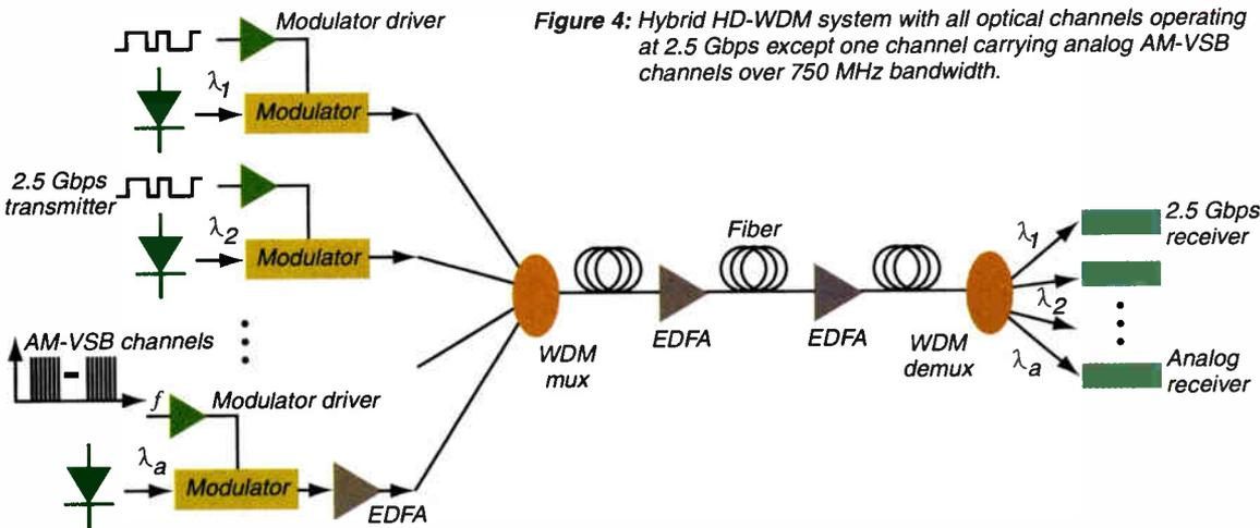
Figure 4: Hybrid HD-WDM system with all optical channels operating at 2.5 Gbps except one channel carrying analog AM-VSB channels over 750 MHz bandwidth.
