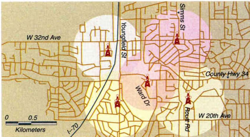
**Figure 1: Coverage map.** In a test over TCI facilities in Lakewood, Colo., PCS Solutions' CMIs delivered robust signals over four coverage areas measuring 2,000 feet in radius, and one, located on a small hill, measuring 2,500 feet.
