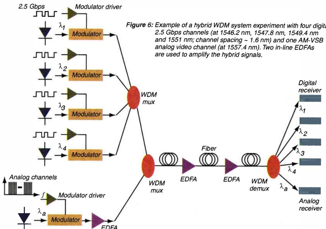
Figure 6: Example of a hybrid WDM system experiment with four digital 2.5 Gbps channels (at 1546.2 nm, 1547.8 nm, 1549.4 nm and 1551 nm; channel spacing ~1.6 nm) and one AM-VSB analog video channel (at 1557.4 nm). Two in-line EDFAs are used to amplify the hybrid signals.
