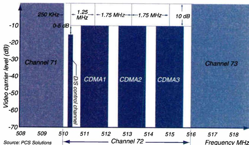
**Figure 2: Downstream signal allocation. Three 1.25-MHz CDMA channels are positioned within the 6 MHz downstream and upstream channels of the cable network as indicated (also see Figure 3). CMIs modulate outgoing signals to the 1.9 GHz PCS frequency, and incoming frequencies to the cable channel levels.**
