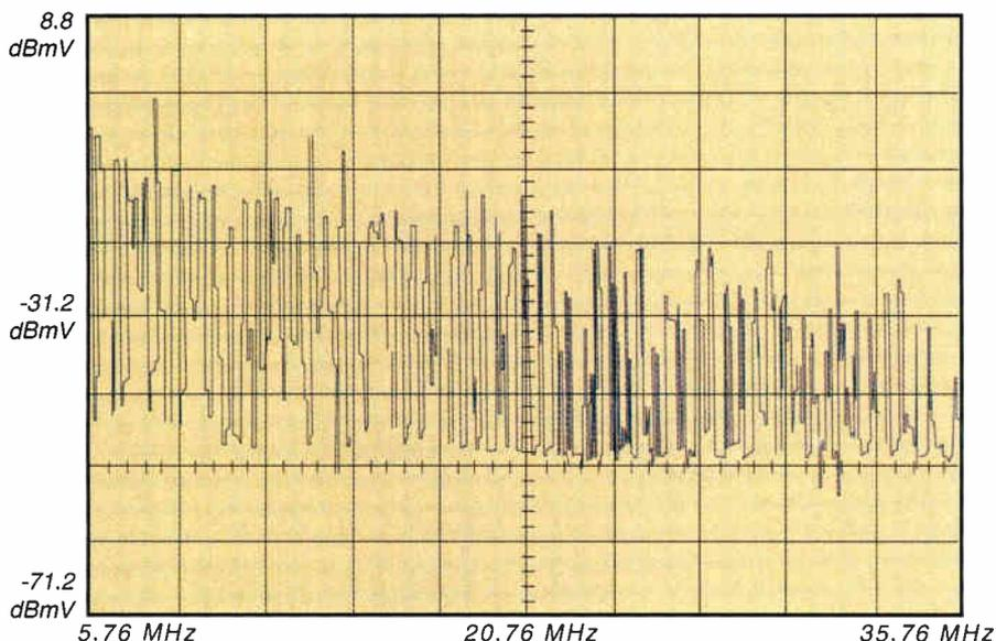
this article. The premise of the test involves a primary carrier at 8 MHz which is increased in level by 2 dB steps at the input to the return laser until the second (16 MHz) and third (24 MHz) harmonics appear, indicating clipping in the laser. The viewed harmonics could come from single-ended return amplifiers. However, the amplifier input range is generally greater than the laser and not the source of the harmonics. In short, the laser will most likely be the source of the problem.
