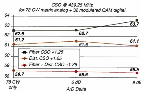
Figure 7: 50-550 MHz analog tier XMod data comparison
