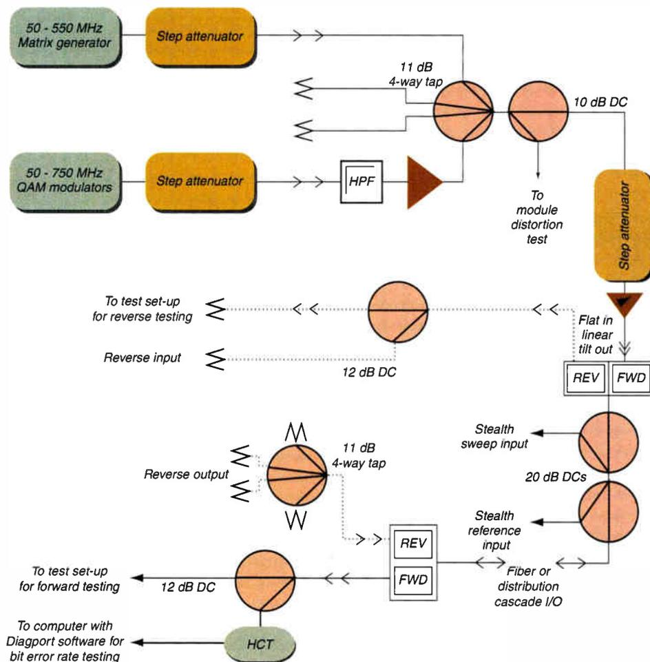
The tests performed were to determine what effect the digital tier (550 - 750 MHz) had on the analog tier (50 - 550 MHz) and what effect the analog tier had on the digital tier. A number of tests were performed to help in determining the effects of noise, distortions and Bit Error Rate (BER).
