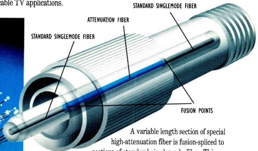
A variable length section of special high-attenuation fiber is fusion-spliced to sections of standard singlemode fiber. This reduces reflections, minimizes cladding effects, and eliminates epoxies from the optical path. It also allows connectors to mate to standard fiber.
