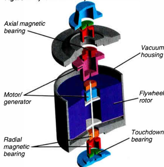
Figure 2: Flywheel installation.
