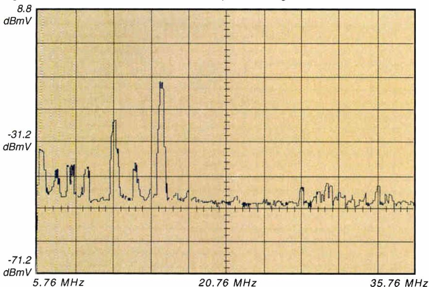
is a tone sequence equally divided on each side of a center frequency and appearing as though it represented the peak power level of a form of QPSK modulation. The testing was run on an active network, and the results
