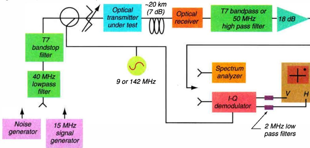
Figure 5: Notched noise plus CW carrier.
