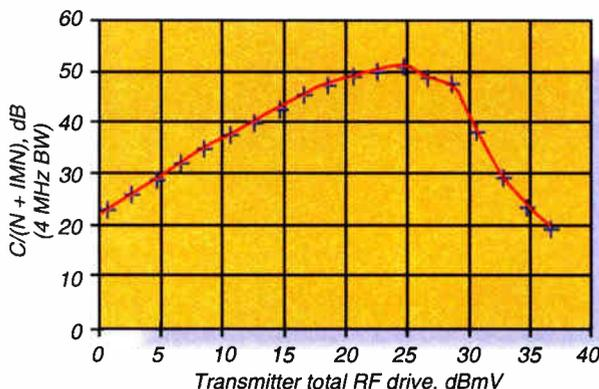
Figure 7: Laser 2, +1 dBm, isolated, uncooled DFB.
