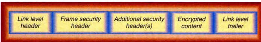
Figure 3: Encrypted HFC frame security header
