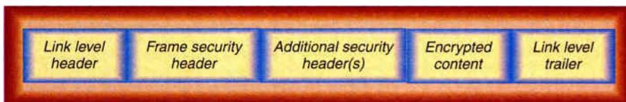
**Figure 3:** Encrypted HFC frame security header
