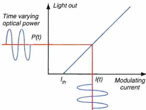
Figure 3: Laser light output when the OMI is greater than 100 percent.
