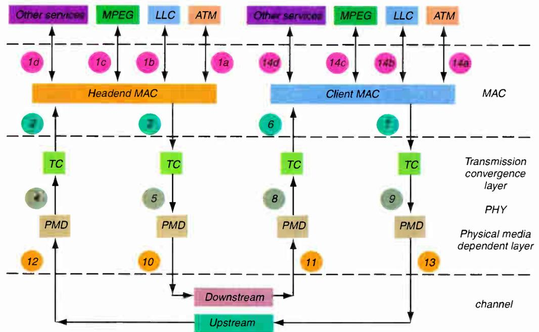
Figure 2: IEEE 802.14 upstream channel model
