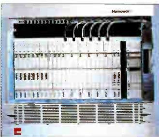
ADC's Host Digital Terminal supports 28 DS-1 or 24 E-1 inputs.
