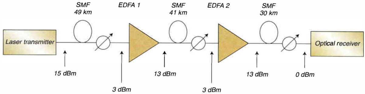
measured CNR (channel 78) was 53.7 dB with CTB distortion less than -65 dBc and CSO distortion less than -70 dBc. In order to select the proper operating point of the AM/QAM video lightwave trunking system with the cascaded EDFAs, the optical input power to each in-line EDFA needs to be determined.
