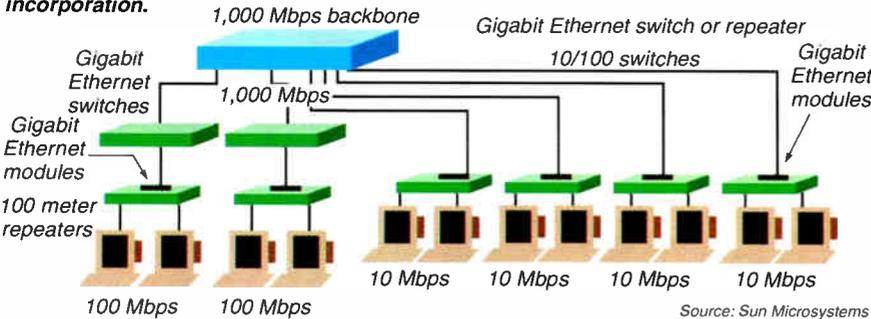
Switched fast Ethernet backbone network after Gigabit Ethernet incorporation.
