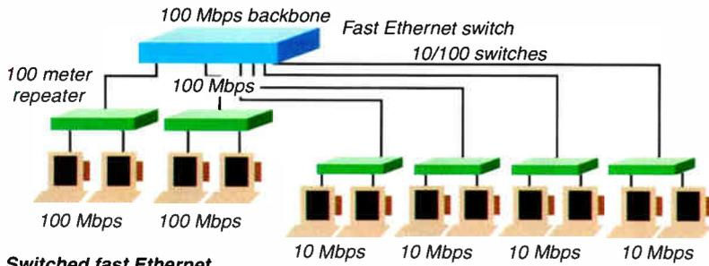
Switched fast Ethernet backbone network prior to Gigabit Ethernet incorporation.
