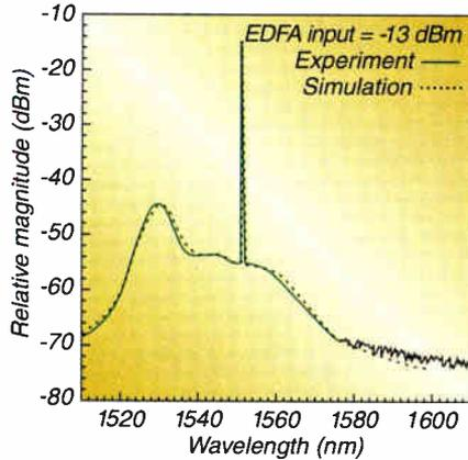
EM-DFB laser transmitter with three cascaded 980-nm pumped EDFAs and a standard singlemode fiber (SMF).<sup>13</sup>
