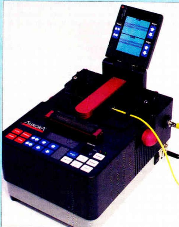
BLUE BELL, Pa.—Aurora Instruments Inc. has introduced a new fiber optic fusion splicer, the Fusion 2500. Having a wide-angle viewing video monitor on an omni-directional swivel mount, the Fusion 2500 shows two simultaneous 65X views of the fiber. A video output port allows the user to display the fiber images on an external monitor as well. The splicer also utilizes Aurora's core-to-core alignment system to produce low splice loss-
