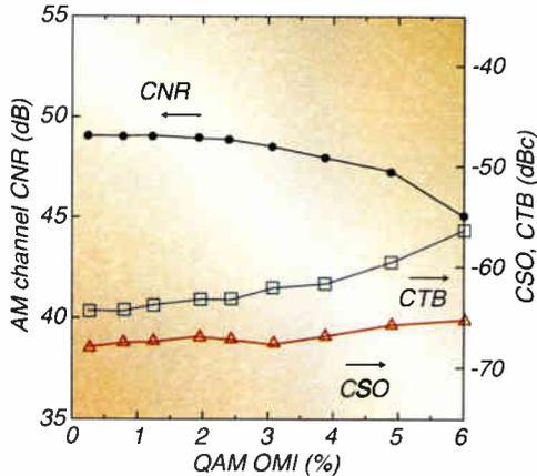
a high-power in-line EDFA should be 5 dB or less when operating deep in saturation for high performance AM video lightwave trunking links. An AM CNR greater than 50 dB with CSO and CTB distortions less than -65 dBc, and nearly error-free transmission (uncoded BER  $\leq 10^{-9}$ ) for the 64-QAM channels with SNR of 30 dB or better has been achieved.
