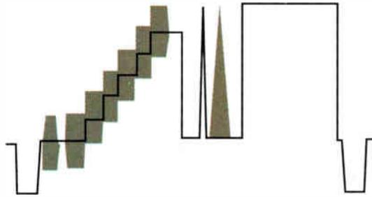
**Figure 4:** The NTC7 composite signal has some limitations for making color tests because its staircase exceeds 100 IRE and can cause a properly adjusted modulator to momentarily overmodulate.
