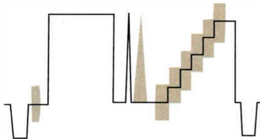
system, and the time it takes for the black-and-white portion of the signal (luminance) to pass through a system. The amount of distortion is expressed in time in nanoseconds. If the number is positive, the chrominance is slower than the luminance. If the number is negative, the chrominance is faster.
