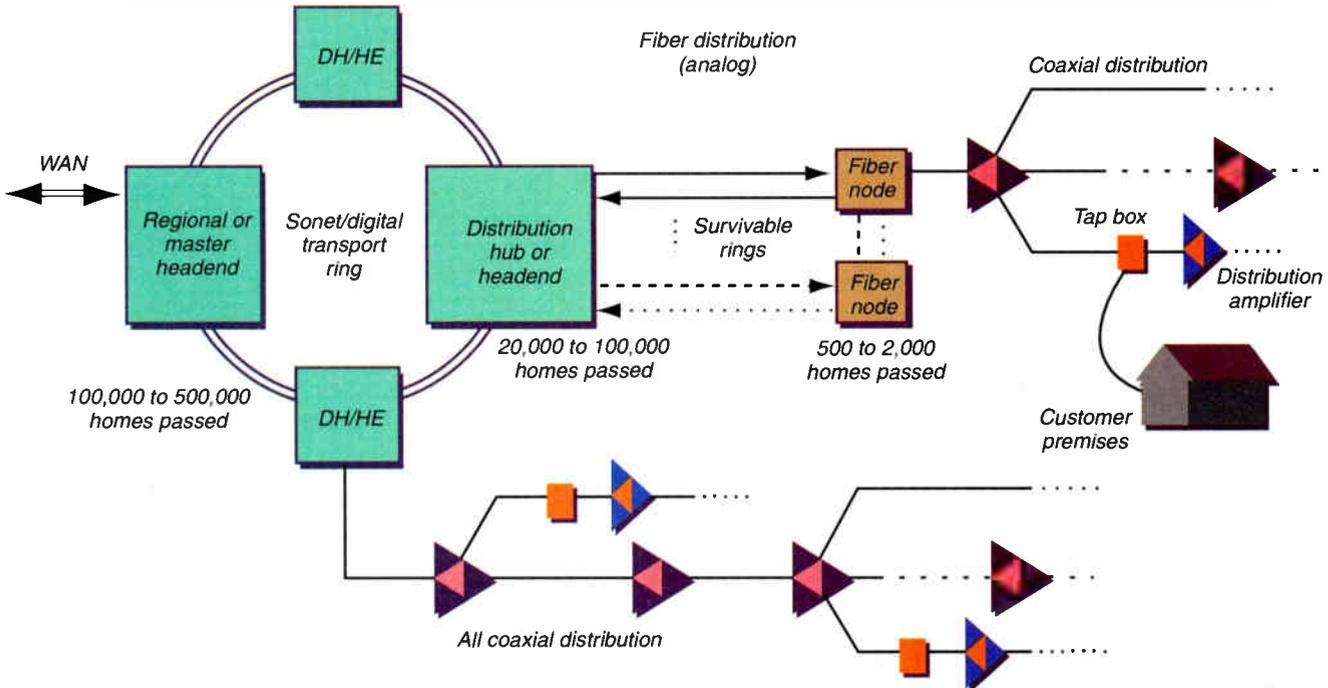
information to and from the subscriber. These RF channels are located in available channels in the forward spectrum, typically between 50 MHz and 550 MHz. In the reverse direction, RF channels bringing data back from the subscriber are generally situated in the 5 MHz to 30 MHz range. Newer and upgraded hybrid fiber/coax (HFC) cable systems are generally designed to extend the forward spectrum to 750 MHz and the reverse to 42 MHz.
