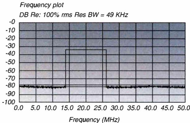
also limited by distortion. However, in most reverse path optical links, the laser dynamic range is so small that this distortion is because of laser clipping.
