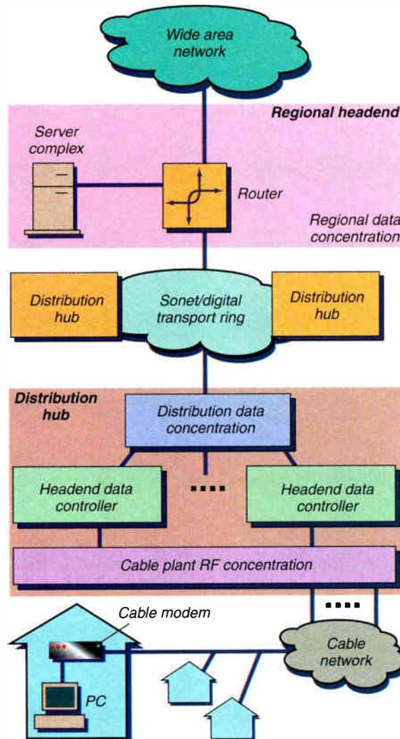
Figure 4: Node aggregation within distribution hub
