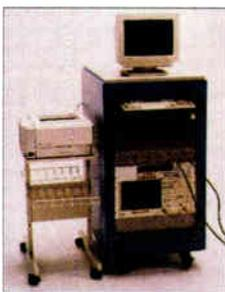
DCM's coaxial cable measurement system
