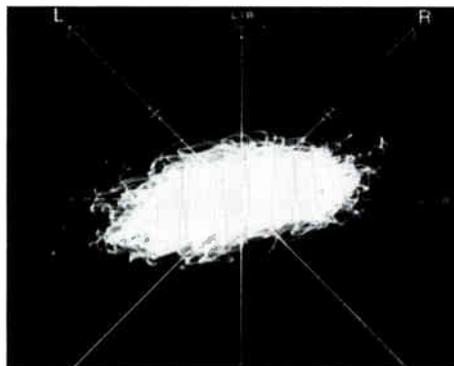
Figure 3: Out-of-phase stereo, unsuited for mono.
