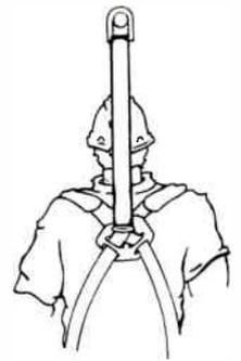
**Full body harness (L2000-ESP) developed by Essential Safety Products and DBI/SALA. It's designed to be worn throughout the day, if needed.**
