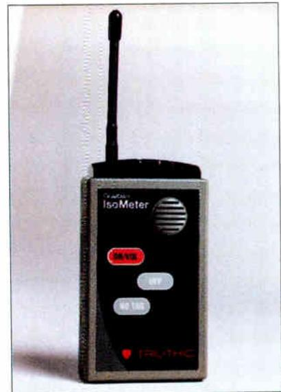
**Trilithic's reverse leakage detector**
