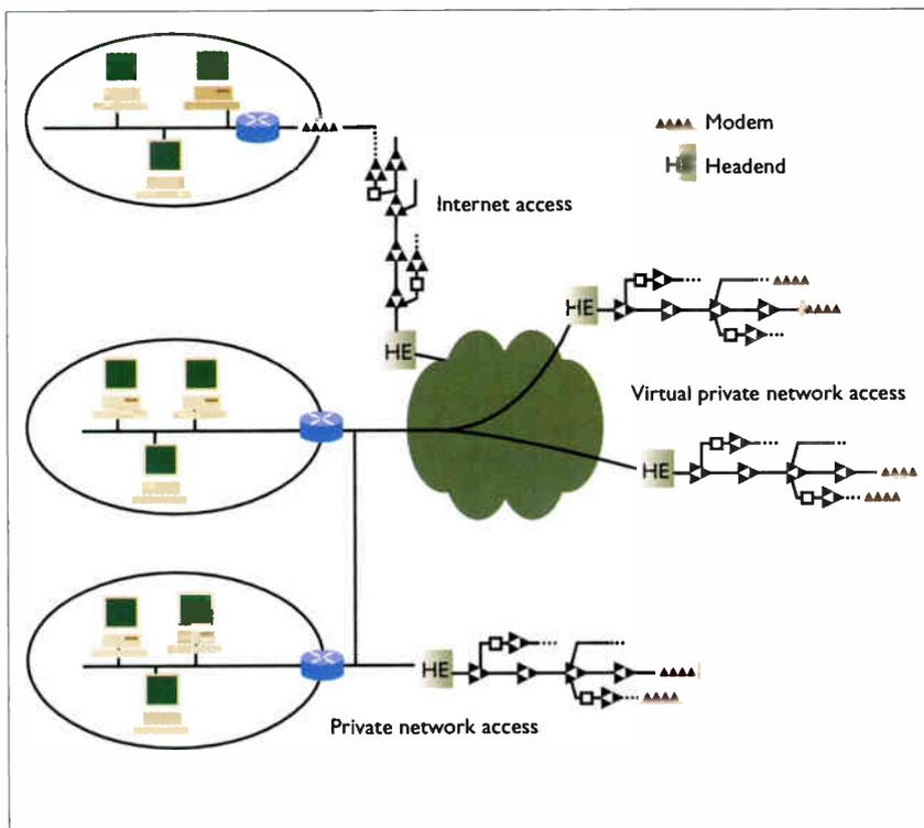
Figure 1: Three types of access supported by the cable infrastructure: the Internet, private network and virtual private network—all of which connect end users to the respective networks through their headends. The virtual private network is represented by a private network and secured “tunnels” within the public Internet.
