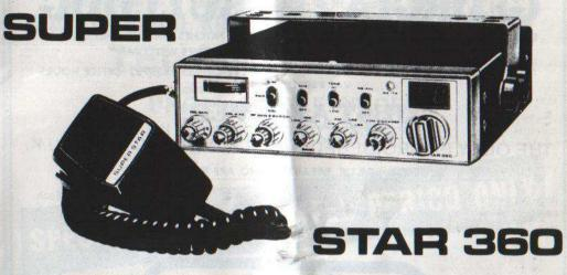
General Specifications: Channels 120 AM, 120 USB, 120 LSB and 120 CW. The Frequency Range is 26,965 to 28,940 MHz, with Frequency Tolerance at 0.005% and Frequency Stability of 0.001%, Overall Cabinet dimensions are 203mm W. x 64mm H. x 235mm D. The meter is illuminated and indicates relative RF power output and SWR on Transmit, received signal strength.
