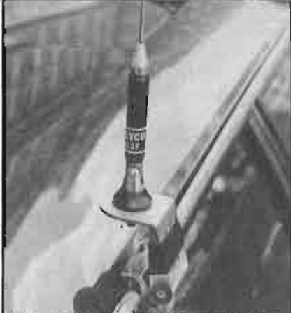
Above: Gutter mounting means no drilling, but cable run can be untidy. Below: Boot mount—simple but sites are limited.
