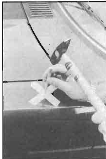
Above: Marking panel to be drilled with tape protects paint when drilling. Below: Centrepunch at centre of cross to stop drill skidding.
