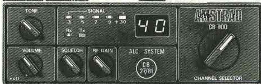
Amstrad CB900 Rig. Highly advanced rig with squelch control, RF gain, LED "pound" meter, ALC system, tone control and LED transmit/receive displays. Note the CB 27/81 Certificate of Compliance symbol.
