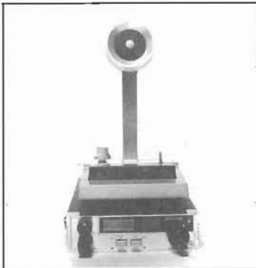
The rotary knobs on this AudioLine rig have been replaced with flats. They also stand out half an inch from the face of the rig, making them easier to turn.
