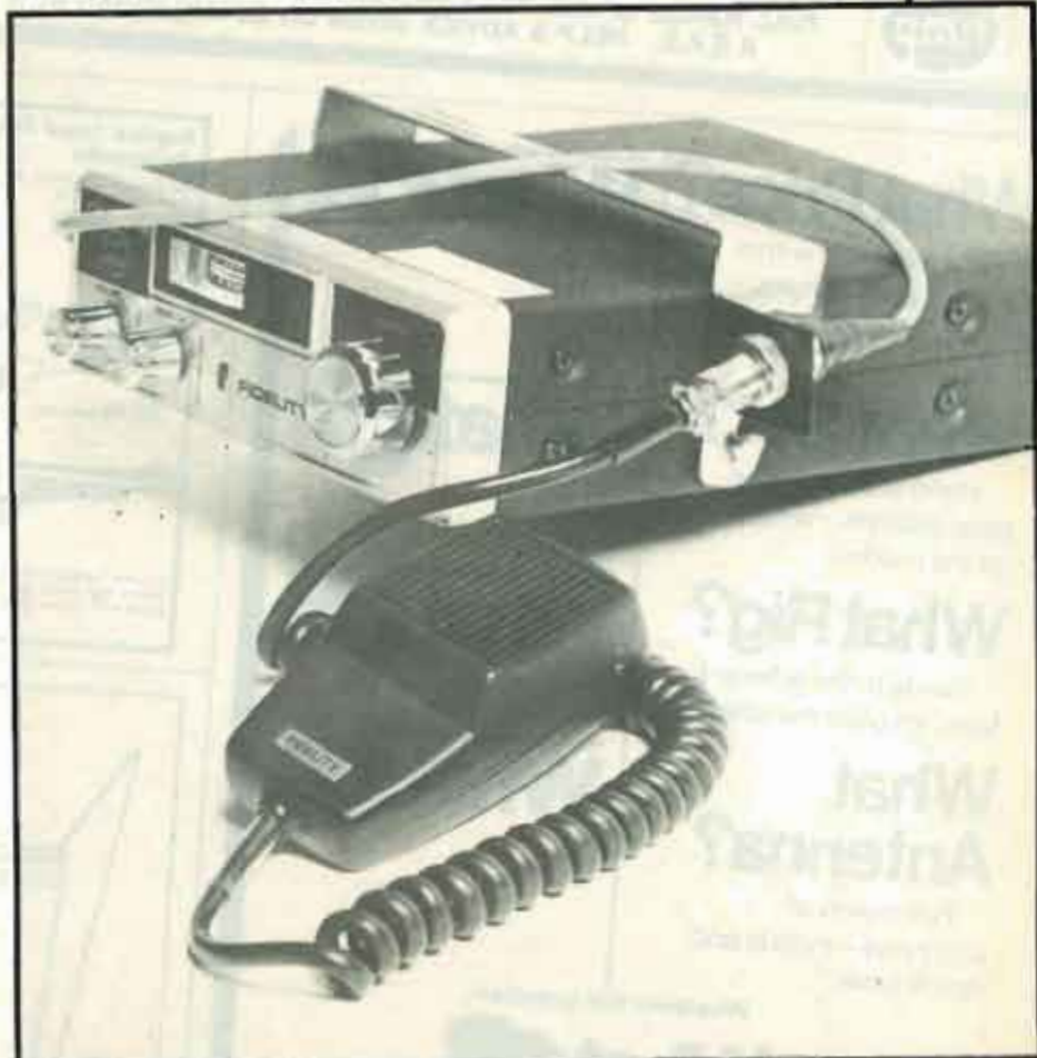
The complete lead with four pin plug and socket
