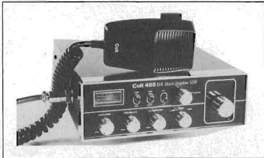
Above: Not so much the big brother of the Colt 295, this must be its grandfather. The Colt 485 DX Black Shadow SSB has AM, upper and lower sideband with high and low channels, giving a grand total of 240. As well as refinements like PA and a noise blander, the 485 has a clarifier which is of real use with an SSB set. The cost, if you could find one, would be around £150.
