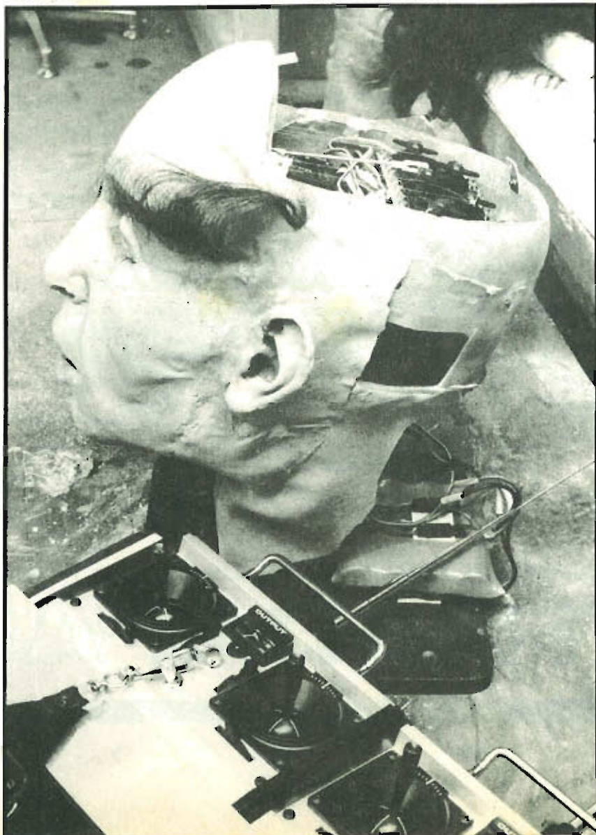
A head for figures. The top of the head lifts off with the wig (below) to give access to five of the servos and two receivers (above). The wiring acts as an arriel.
