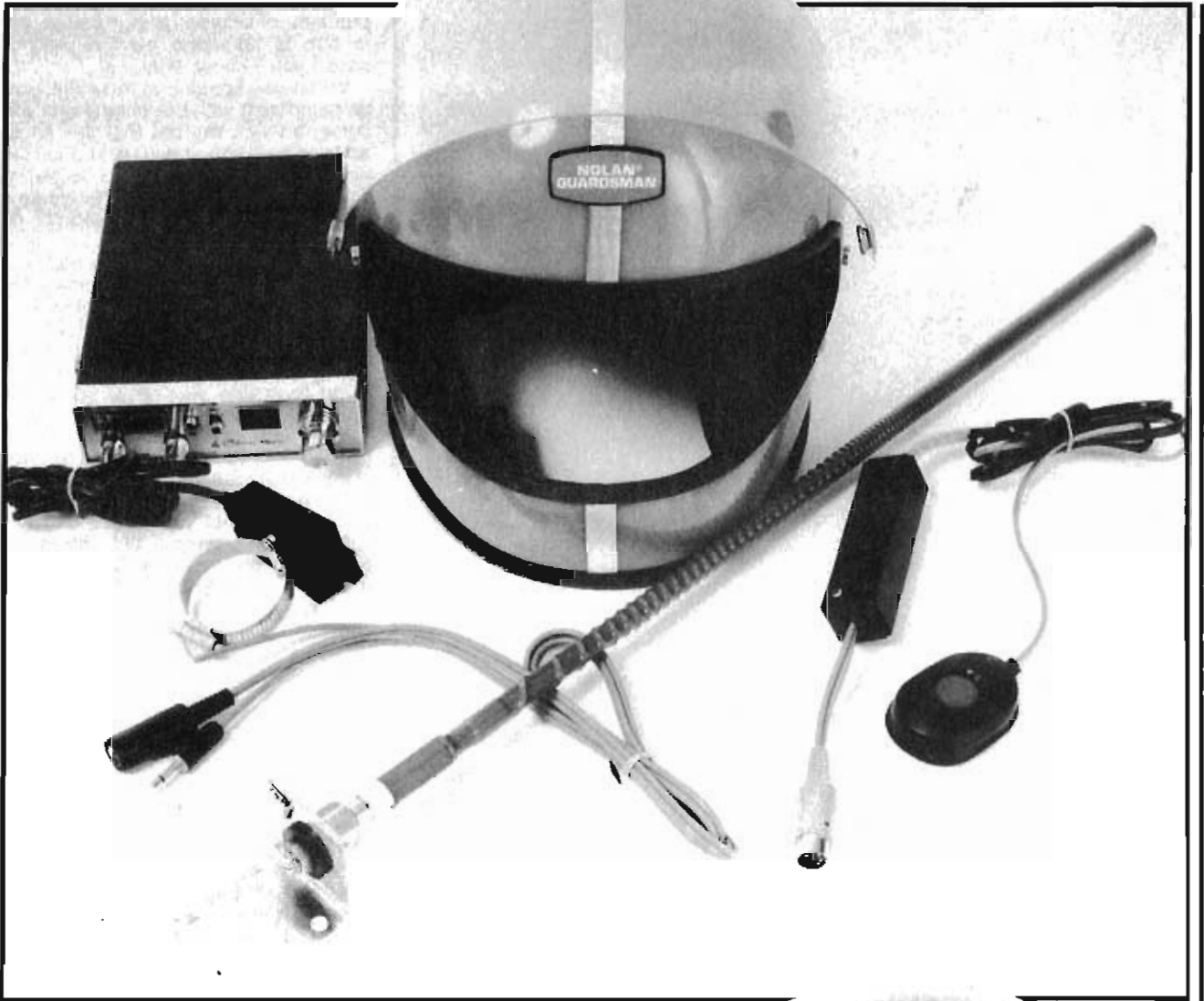
A closer look at the equipment. Above is the full kit for the full face including the Superex mike, speaker, push-to-talk control and quick-release connections. The antenna is from the Frestik mirror-mount dual twig kit. We used a Cobra 19GTL rig but any compact unit will do the job — just measure up the fairing before you go shopping. Pictured right is the Superex open face kit. The boot is optional.
