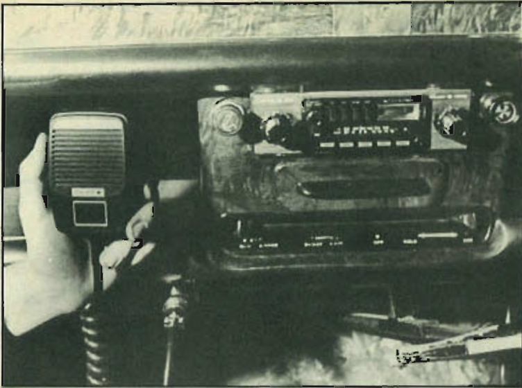
7. The ultimate CB radio: a Cobra set with AM/FM stereo radio receiver plus 40 channel rig with squelch and digital read out on clip-on microphone.
