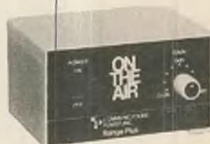
**RP-1** Breathes weak signal life into older sets w/13 dB boost and negligible added noise. Also gives needed strong signal overload protection w/manual gain control. Automatic transmit bypass stays in antenna line rated at 400W. An off-the-shelf item. No tools, no set alterations, just add on. 12VDC.
