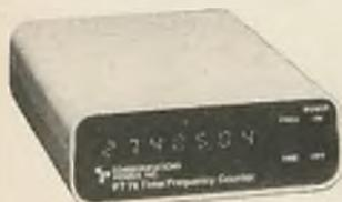
**FF-76** Versatile, feature-filled, 7 digit counter reads 10MHz to 40 MHz or functions as 12/24 hour clock. Quartz crystal reference for remarkable 3PPM stability. Rated at 400W, can remain in antenna circuit. Also has 50MV output for lab/technician use. 12VDC. Also available without clock feature (FC-70). Optional adaptor (FA-70) for receive frequency readout, certain radios including all CPI units.
