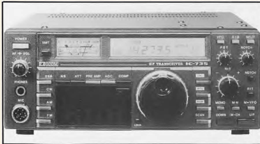
Amateur rigs such as Icom's IC-735 are easily converted to cover 11 metres FM.
