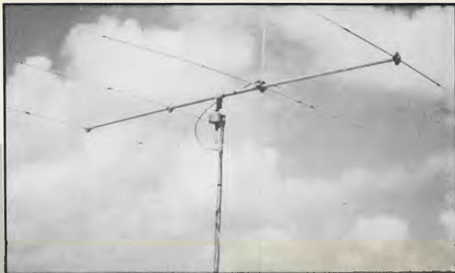
Four element, dual polarity, Yagi does a nice job for the group.
