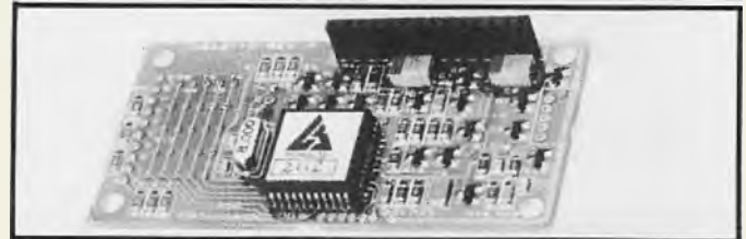
Above: Selcall module for Philips FM620 measures just 80mm x 40mm x 10mm while five tone sequential encoder/decoder shown below measures slightly smaller 50mm x 37mm x 6mm. Both are produced by GSA Technology Pty Ltd.
