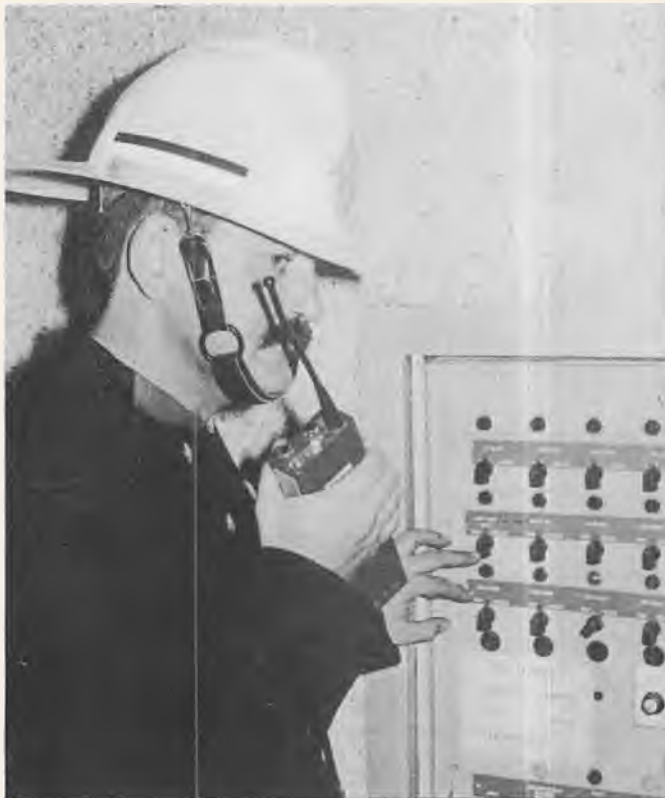
A NSW fireman checks a building fire alarm, and uses a Motorola MX-350 UHF handheld to 'crossband' back to headquarters via his VHF mobile.
