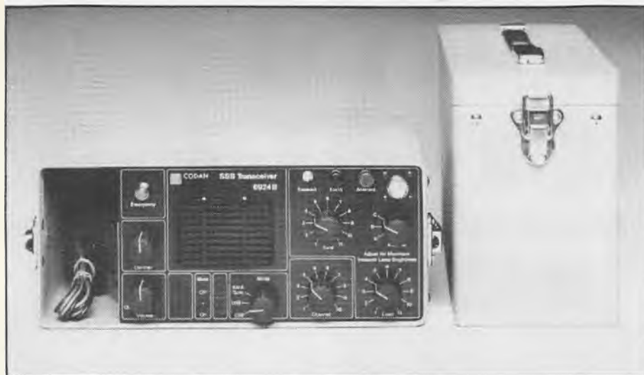
This Codan HF SSB rig is popular with travellers who need reliable long distance communications in the outback.
