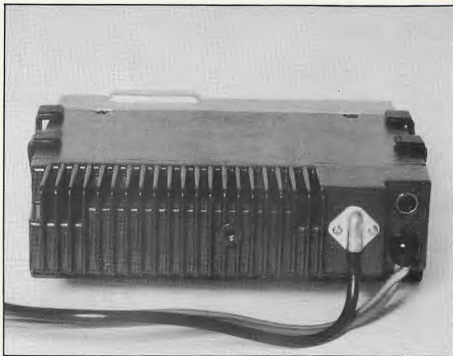
999 uses flying leads instead of fixed connector sockets on the rear panel which makes installation easier than with most CB rigs.
