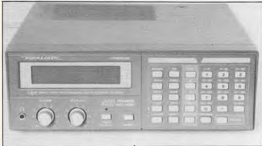
New PRO 2006 resembles the 2005 but introduces the accelerated scanning technique 'hyperscan' — 26 channels per second on fast scan and 13 on slow.
