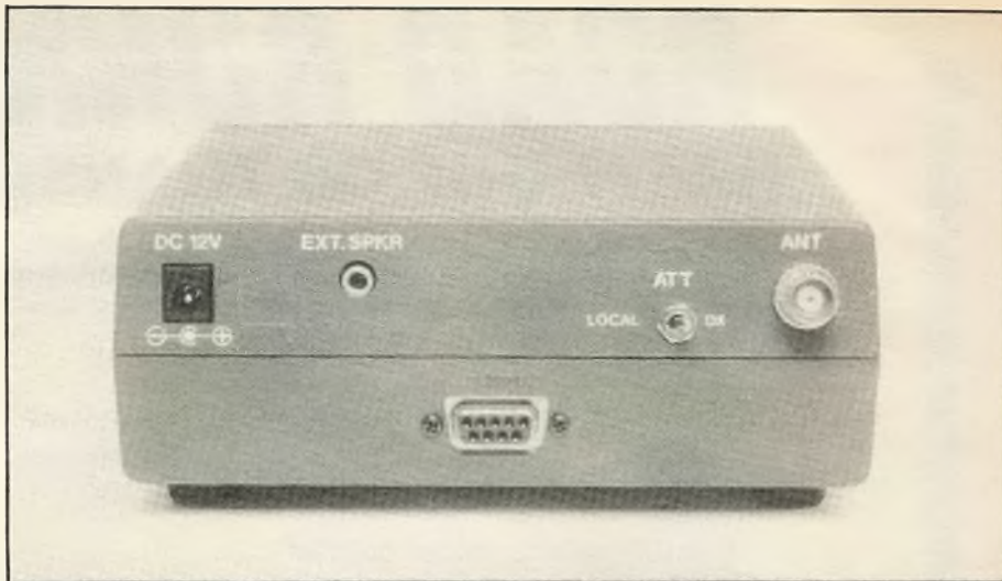
Rear panel has BNC connector, attenuator switch, RS232 port, DC socket and extension speaker jack.
