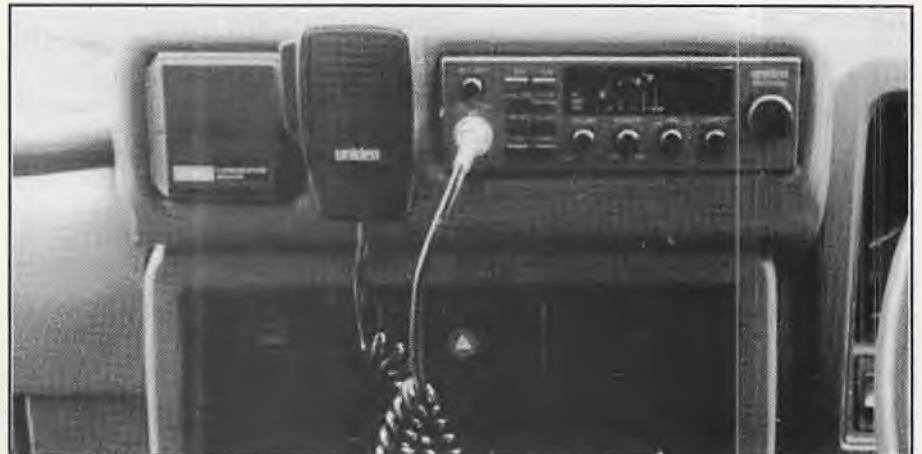
Above: Rig fits neatly into after-market accessory panel in Nissan Patrol.
